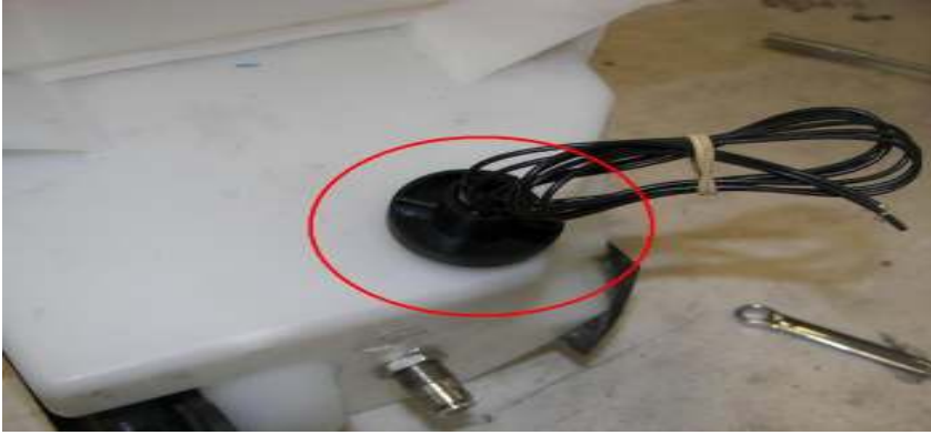
Fluid level switch and Bulkhead fitting shown on '07 Mustang Washer Bottle.
