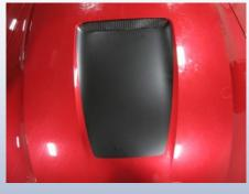
Vinyl that needs to conform to curves of the hood can be pressed into place with your hands or if need be the use of a hair dryer to help conform to the shape of the car. Also when tucking vinyl around the edges of the car. **Do not over heat it will shrivel or wrin-kle.**
