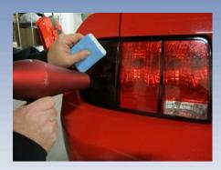
Note from 99-04 put the bottom piece on then the piece that sits on top the brake light. Making sure the first is dry and cooled before doing the second. Then heat the top and with your hands wet roll the top over the bottom.
