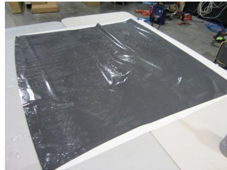
**Step 4:** With the help of an assistant pick the vinyl up and lay it on the roof being careful not to wrinkle the vinyl. This is were being in front or back of the car makes it easier to just grab the vinyl by the corners and basically flip it onto the roof.
