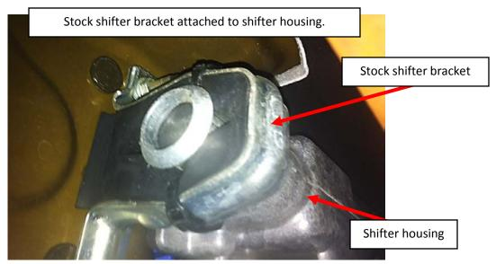
3. Locate the factory shifter bracket. It will look just like the photo above. You will need a 10mm deep socket in order to remove the (2) nuts holding the bracket in place. You might have to tug it a bit for the retaining clip to let it go. Once done, you can pull the factory bracket off the end of the shifter housing. See photo below.
