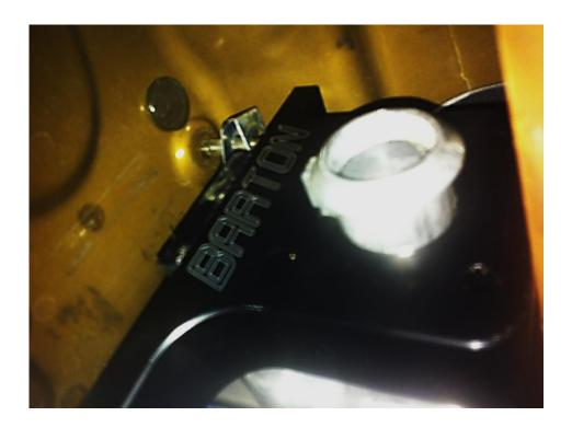
6. Lift up the entire Barton bracket onto the (2) studs and reinstall the (2) 10mm nuts using the deep socket.
