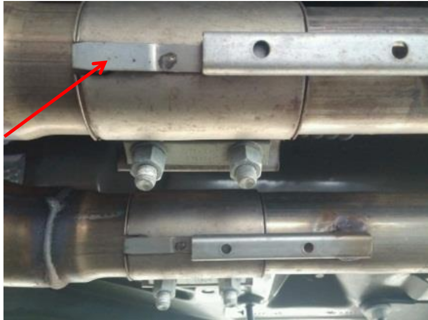
Figure 2 X-pipe Clamp Removal
