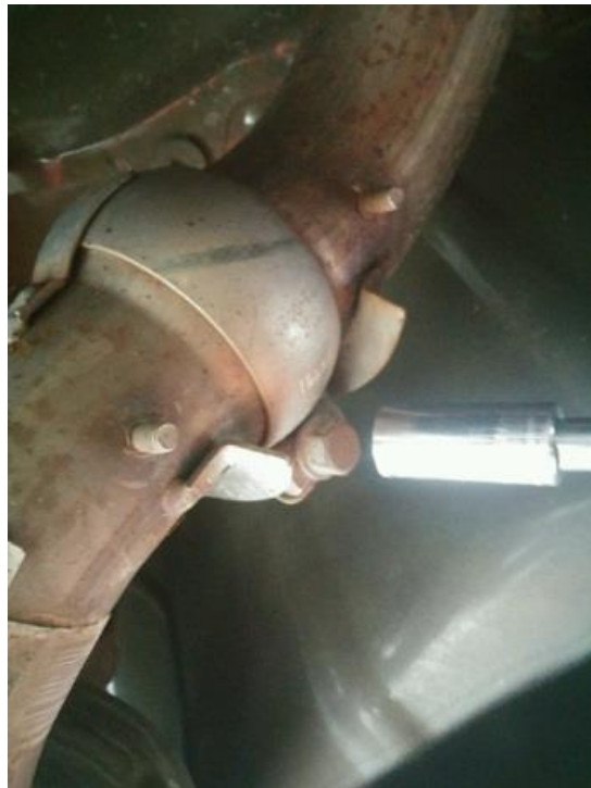
Figure 1 Ball and Socket Clamp Removal
