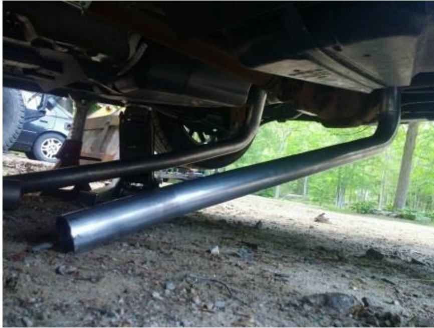
Figure 3 New Over-axle Pipes
