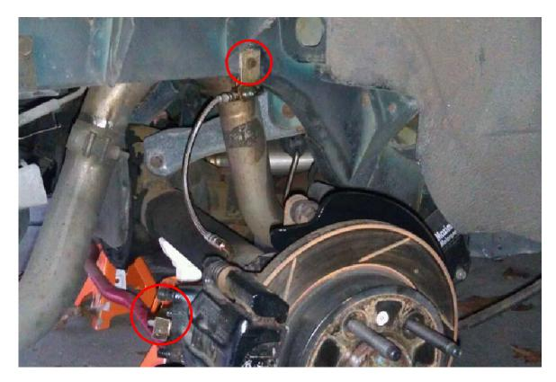
3. Start removing the old rubber brake line. You are going to remove the steel brake lines from the rubber hose. For this installation, I am showing you the passenger side which has (2) steel lines meeting the rubber hose. Take your 13mm wrench and loosen the (2) steel lines all the way until they come off the junction. They are labeled in the following picture with red circles. **NOTE**: brake fluid will slowly drip out but not enough to clear the system.
