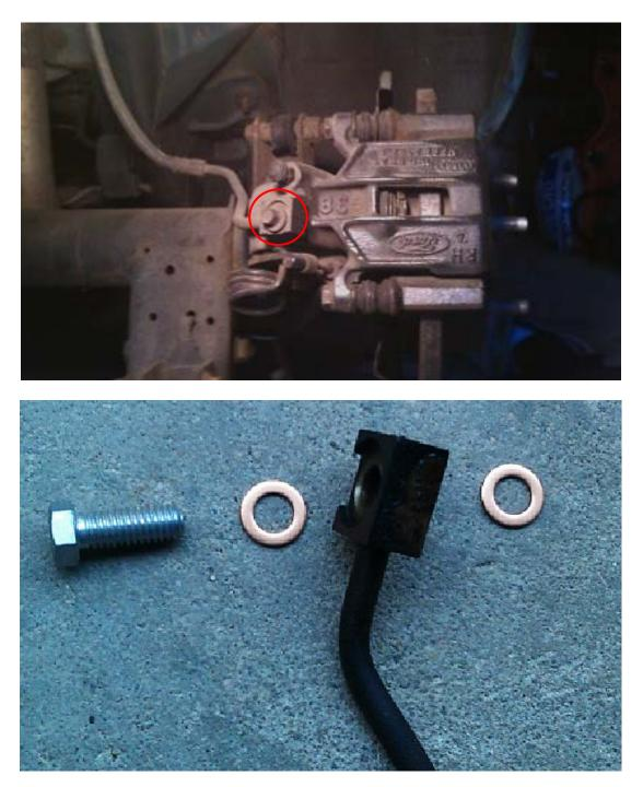
6. Now it's time to install your new lines. You are going to work in the same order as removal. Start by installing your existing steel lines into the junction block of the new stainless steel hose. Make sure you start the fittings by hand because they strip out very easy. Once they are started by hand, finish tightening them with the 13mm wrench. It should then look like the following image.
