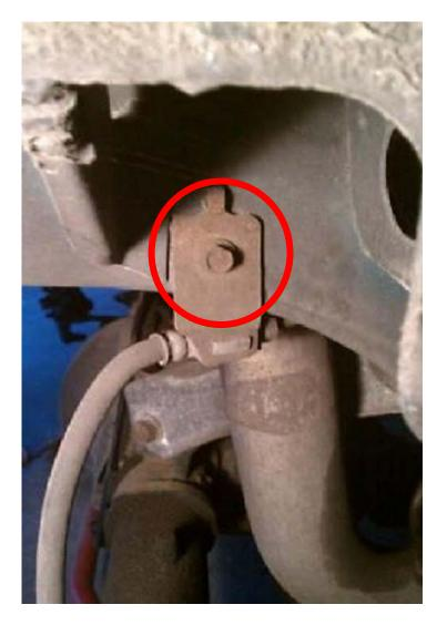
5. Now remove the line from the caliper. The banjo bolt is 10mm so use your ratchet to remove it. Once removed, you will then find (2) copper washers. One between the head of the bolt and the line and the other between the line and the caliper. You will need to keep this order when you install the new line; however, you will need to replace the washers with new ones available at any local auto parts store. The photos below show the location of the banjo bolt as well as the order of the parts.
