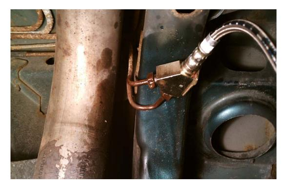
7. Take the self-tapping bolt and bolt the hose bracket to the same place on the body as the old one. Use your 10mm socket and tighten it down.
