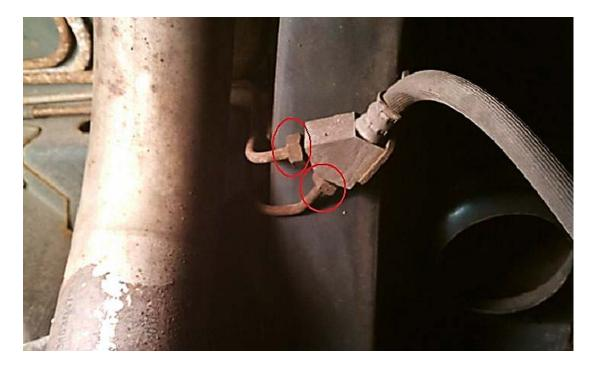
4. Take your ratchet and 10mm socket and remove the (1) mounting screw holding the bracket to the frame circled in the following picture. Be sure to keep the screw to reuse when you install the new brake lines.
