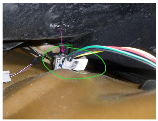
**4)** The Raxiom sequencer will go in between where the wires are currently clipped together (like an extension cord of sorts). Attach each side of the Raxiom sequencer to the cables you just unclipped (shown in green). Repeat for the other side.
