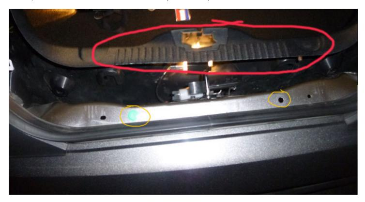
**3)** After sliding out the plastic piece, you should see the taillight connectors (in green) near the back of each of the tail lights. Push on the release tab and disconnect the connector.
