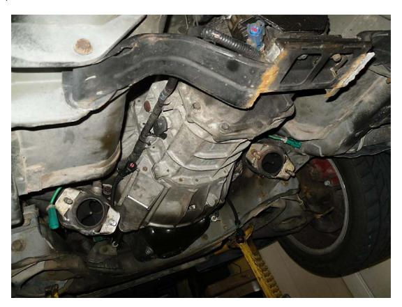
7. Unbolt the transmission mount from the cross member by removing the (2) 18mm bolts.
