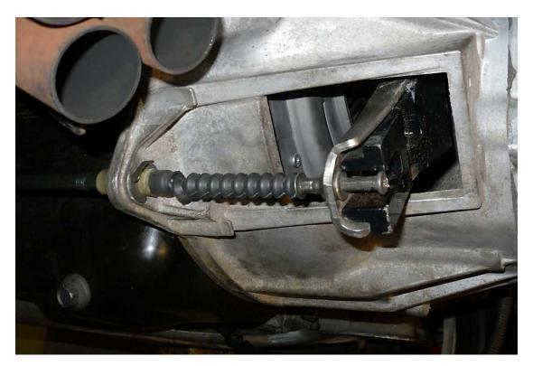
25. Attach the clutch cable dust shield with the 8mm bolt removed earlier.
