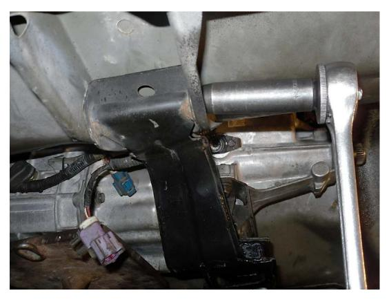
29. Slide your driveshaft back into place in your transmission and then install the (4) 12mm bolts removed earlier with a wrench.
