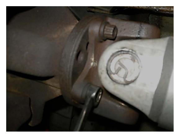
4. Once all bolts are removed, slide your driveshaft toward the rear and remove it from the transmission.
