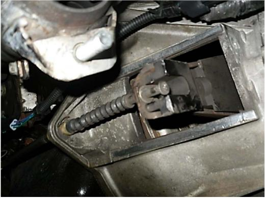
13. Push the clutch fork toward the front of the car and slide the cable off the fork. Then remove the little c-clip against the transmission wall and slide the clutch cable out of the transmission hole so it is free hanging and not connected to anything.
