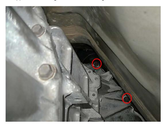
24. Reinstall your clutch cable on your transmission by pulling it through the transmission wall onto your clutch fork. Put the c-clip back on where the cable goes through the transmission.
