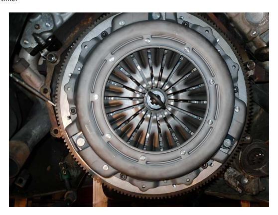
21. Be sure the clutch goes through all (3) dowel pins on the flywheel and everything is aligned before you tighten the (6) 12mm bolts completely. Torque bolts to 30 ft/lbs.
