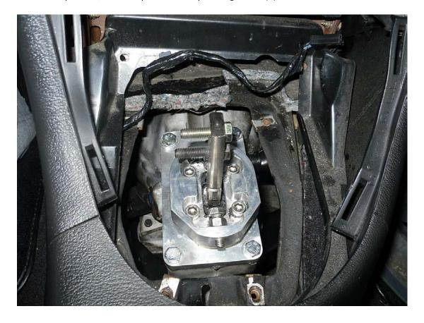
32. Reinstall your boot retainer with the (4) 8mm bolts and slide your shifter bezel over the shifter. Screw on your shift knob.
