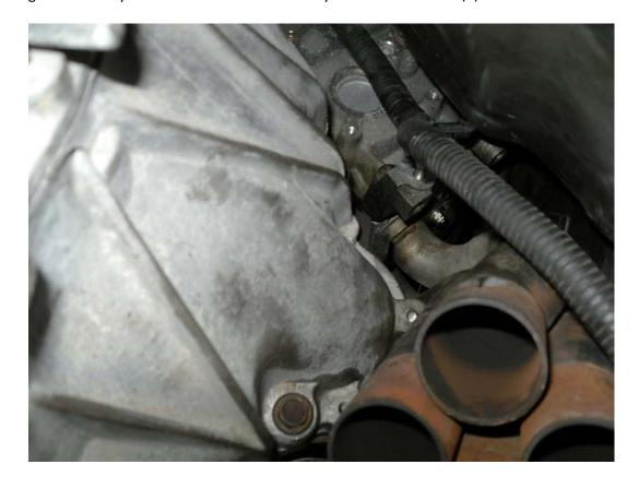
23. Reinstall the (7) 15mm bolts holding the transmission to the engine.
