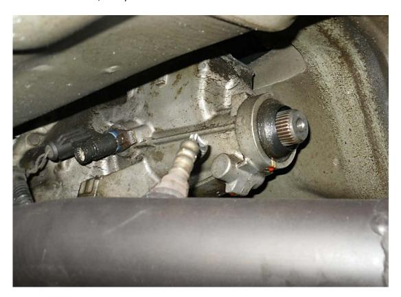
5. Remove your mid pipe by unbolting the (8) 15mm bolts with either a ratchet or wrench (whatever may be easier to use for your particular exhaust) that connect to each of your headers and flow tubes. Disconnect all oxygen sensors and remove your mid pipe.
