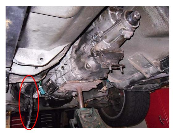
15. Unbolt your starter by removing the (3) 13mm bolts holding it to your transmission. You may need to access these bolts from the front of the car rather than by the transmission. Then remove the (7) 15mm bolts that hold your transmission to your engine; there are (2) bolts on the passenger side, (3) bolts on the driver side and (2) bolts on the top. To reach the top bolts, allow your engine and transmission to sag down a little and use a swivel
