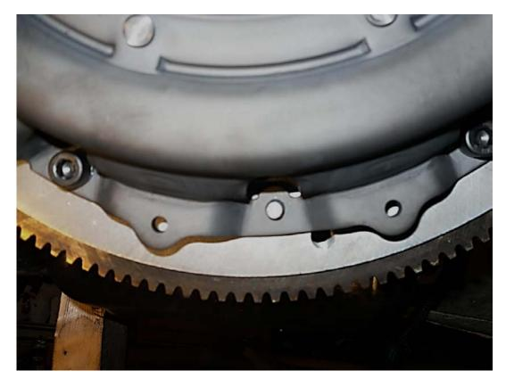
22. Now you can reinstall your transmission. Lift up your transmission and slide it into place in to the clutch; it should go in smoothly so do not force it in. Reinstall your starter with the (3) 13mm bolts removed earlier.
