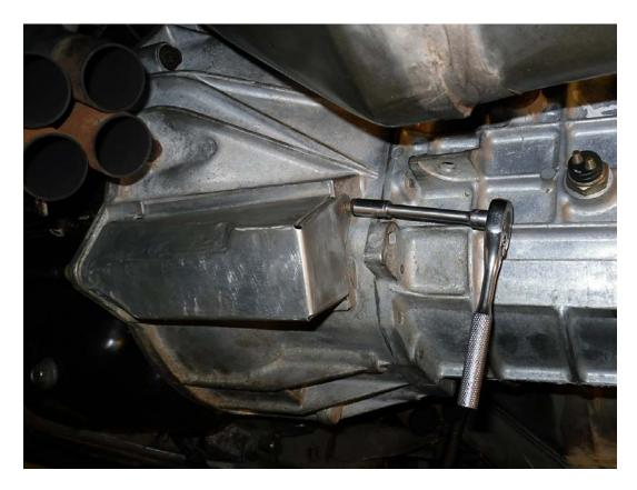
$26. \ \ Connect the \ vehicle \ speed \ sensor \ with \ the \ 10mm \ bolt \ removed \ prior.$
