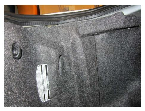
3. Once you have removed all the panel retainers you can start to wiggle the panel out of place, I found it easiest to slide the bottom of the panel out rather than the top. Once the panel is free, put it aside in a safe place.
