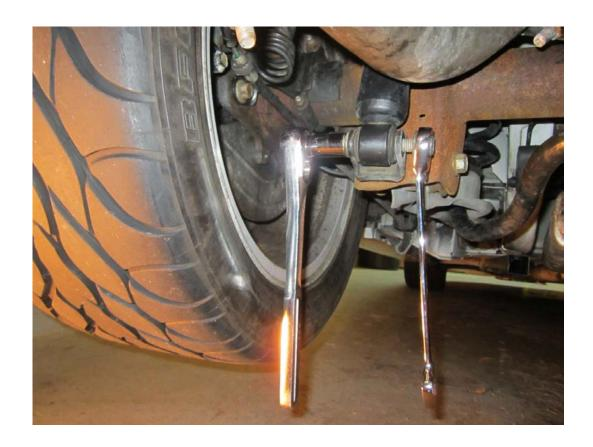
7. Now prepare your new Koni Shocks. This is how the bushing should look when installed on the car; the space in between bushings is where the body will sit.
