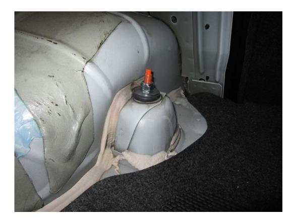
11. Your new Koni Shock is now completely installed; reinstall your truck panel by first sliding it into place than reinstalling all the retainers removed earlier. Push the clip back into place at the seat and the top of the trunk, then twist the retainer on by the taillight. Take your car for a drive and make sure everything feels right. Your Install is now complete!
