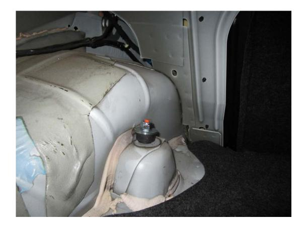
9. Working under the car again, reinstall the bolt and nut removed earlier with your 18mm wrench and 15mm socket. Fully tighten this bolt, then remove the jack and jack stands so the vehicle is flat on the ground.
