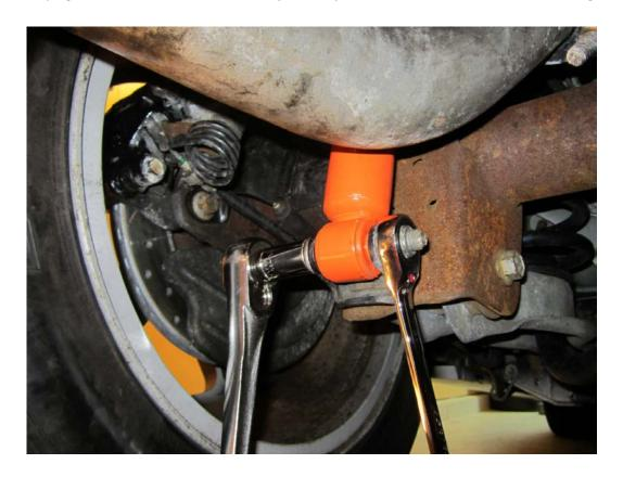
10. Now you must fully tighten the top rear shock mount nut that was started earlier, again it is must easier to use an impact gun to do this however not completely necessary. Use your 19mm deep socket and fully tighten the nut down.
