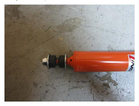
8. Place your new Koni shock into the top shock mount and start the top shock nut first, but do not completely tighten this nut until later.
