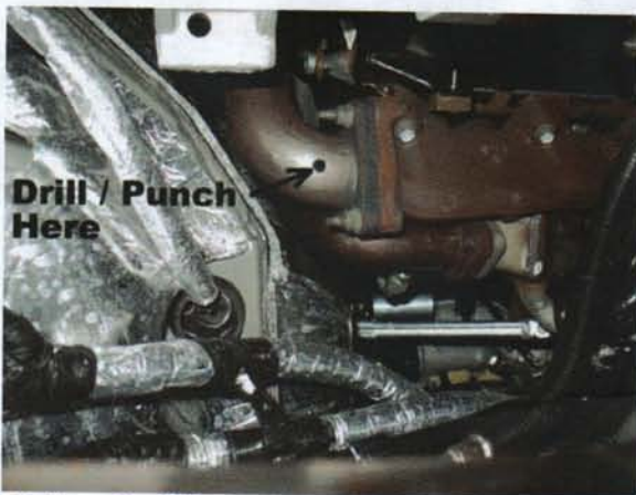
Option 2: This is the preferred location for the EGT sensor. It is also preferred that you punch the hole to 11/32" diameter, rather than drilling. Mark the punch at 11/32" diameter and make sure not to punch the hole any larger than 11/32". You may want to slowly enlarge the hole as you go. Do not drill the hole in this location unless you are proficient in tapping the hole or you may have trouble starting the threads. Drilling and tapping in this location should be left to a professional. You may find it easier to tap the punched hole.
