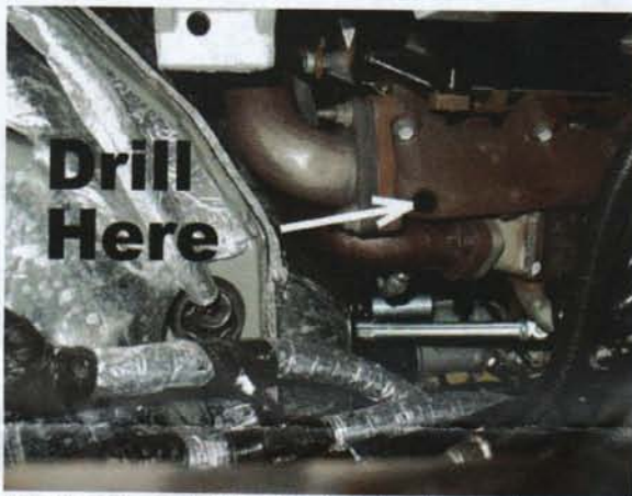
Option 1: Drill the hole into the exhaust Manifold as per the user manual.
