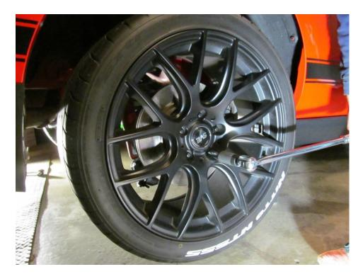
3. Next, jack up the car in the proper location lifting from the rear differential housing in the middle. Place jack stands to suspend the rear of the car on the pinch weld of the vehicle. The rear of the car is being lifted to easily access bolts at each end of the control arm. Once lifted, remove the rear tires.
