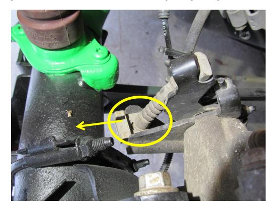
5. Support the rear axle with the jack so when the rear control arms are removed the axle remains in position.
