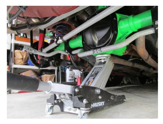
6. With the 18mm socket and breaker bar, loosen the bolts on the front and rear control arms on each side of the vehicle and remove completely. Stock hardware is reused so set it aside. (Drivers side shown)
