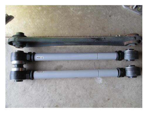
2. Install the RTR Control Arm with the factory hardware. Make sure the large silver part of the control arm bushing is installed at the rear and inside edge.
