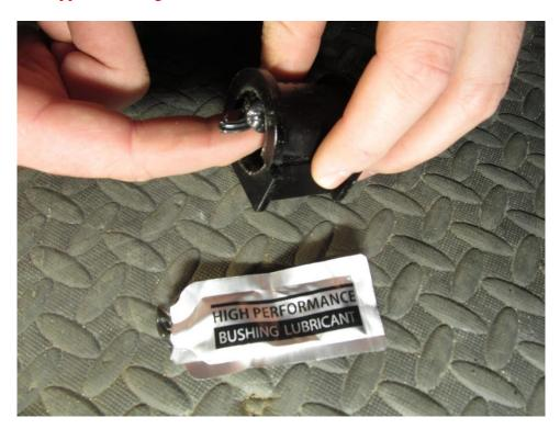
3. Place the bushings on the end of the sway bar and install the lower piece of the axle bracket with the RTR white lettering facing the rear of the car.
