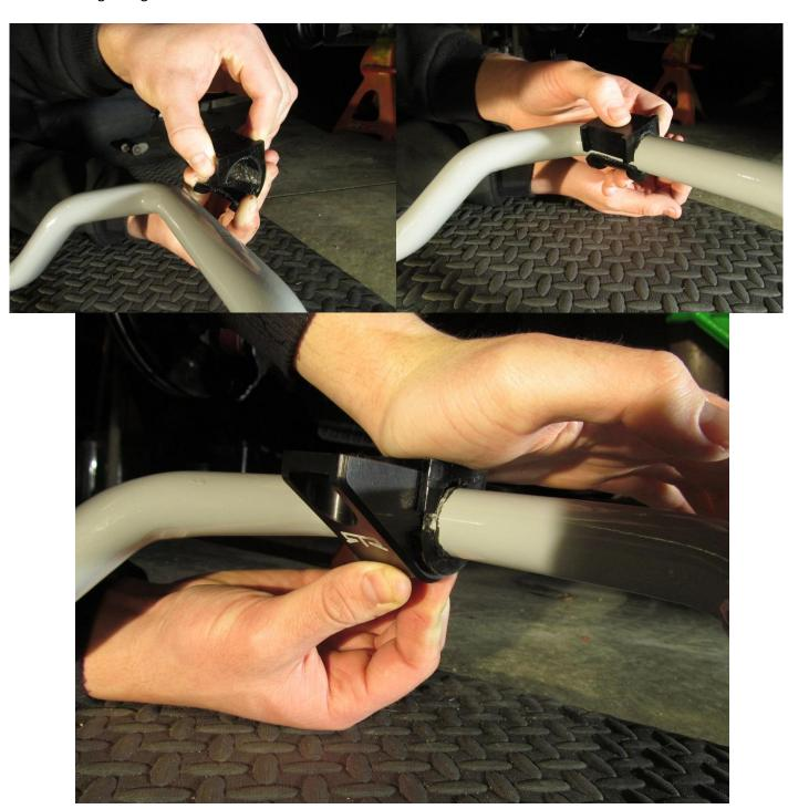
4. From underneath the car put the two other pieces of the axle bracket around the axle and press them in place to hold them in position. Make sure they are even on both sides of the axle.
