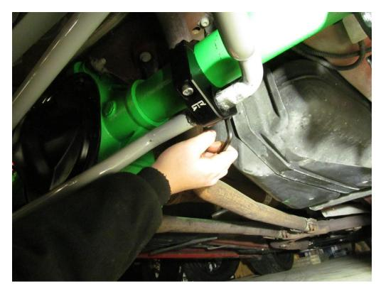
10. The last step is to tighten down the adjustment nuts on the sway bar once they are even lengths with a 0-1 1/2" crescent wrench. Once tight you can install your wheels and lower your car.
