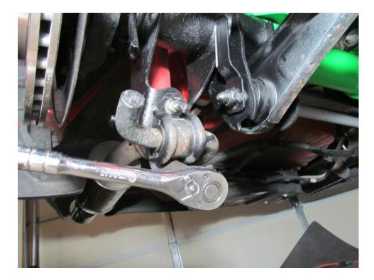
5. The two sway bar links are the only remaining things fixing the factory sway bar to the vehicle. Use the 1/2" drive ratchet and 15mm socket to take off the bolt on the passenger side. Once removed from the passenger side, take the same bolt off of the driver's side. Your factory sway bar is now removed!
