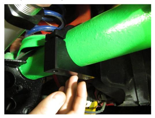
5. With the axle bracket in place, hold up the sway bar and install and snug the bolt using the 8mm allen wrench. The nut does not need to be held because the axle bracket prevents it from turning. In these next steps hand tighten everything until all parts are in place.
