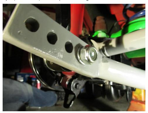
8. With everything now hand tightened and in place use the 1/2" drive ratchet, 19mm and 17mm sockets and wrenches to tighten the sway bar links. The top end of the sway bar link where it attaches to the car can be torqued to manufacturer settings of 86 ft lbs. The lower end of the sway bar link that attached to the sway bar does not have a manufacture specification because the original sway bar link does not attach this way so you will just have to tighten the 17mm bolt to user satisfaction.
