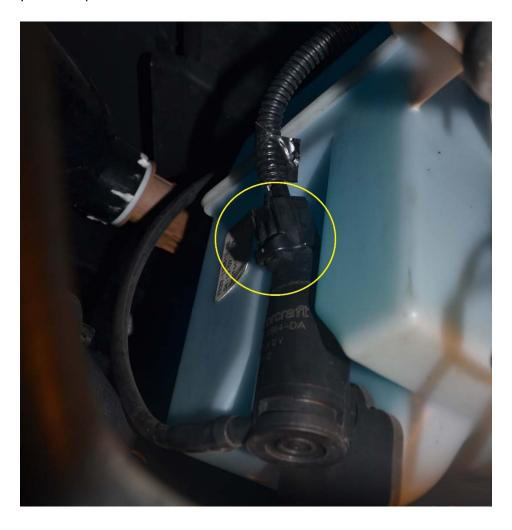
5. Disconnect Windshield Washer Pump Hose, should slide off, and drain the washer fluid in to a drain bucket
