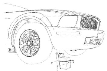
The Windshield Washer Reservoir needs to be removed and installed from underneath the car, will not be able to be access from the top in the engine bay.
