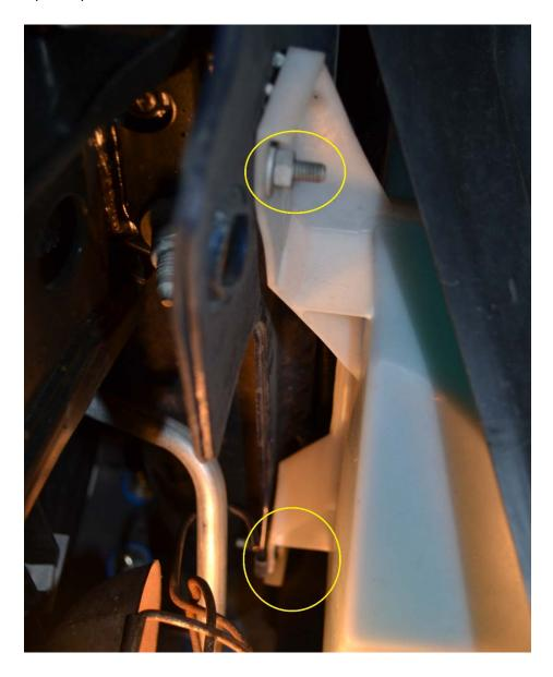
b.  $3^{\rm rd}$  bolt (10mm) is hard to get to, be best to pull back passenger side wheel well liner to access.
