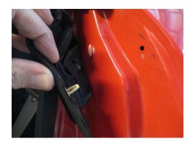
3. Gently separate front and rear molding from lower doorframe.
