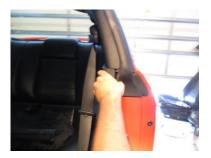
4. Remove old gasket by pinching gasket together and pulling away from vehicle.
