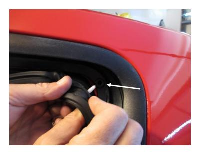
2. Press new gasket into channel and inside interior roof molding.
