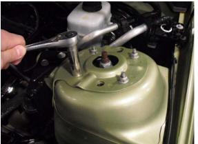
**Step 2:**Place strut bar over strut mount studs and re-install 13mm nuts removed in Step 1.
