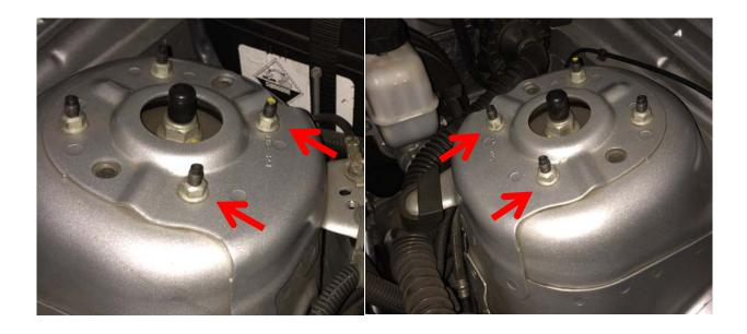
2. Once you remove all four nuts, put the strut tower brace in place, over the strut mount studs, assuring the angled brackets sit flush over the strut mounts (*Note:* If the brace is not sitting flush and angled over the mount, then the brace is sitting backwards)
