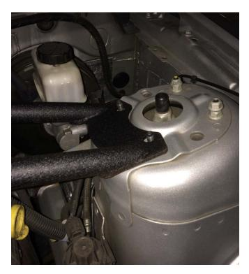
**3.** Screw the nuts back over the brace's bracket; assure they are snug as you will be torqueing them down. Using the torque wrench, torque the screws to 26 ft/lb
