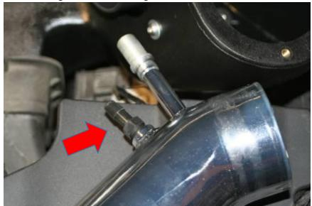
12. Place the mass air sensor into the K&N intake tube and secure with the two screws two 4mm screws using 4mm hex wrench that secure the mass air sensor connection to factory intake.
