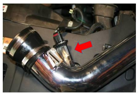
13. Put in the K&N intake tube into the silicone hose at throttle body, then into the silicon hose on the filter adapter. Secure the intake tube with hose clamps by locking the locking tabs with a pair of pliers that secure each hose.
