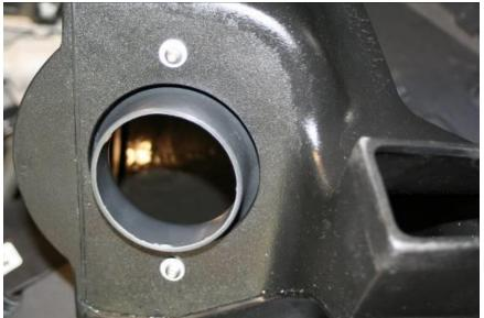
10. Position the K&N air box so the mounting grommets are inserted into the mounting holes and then secure the air box with large screw taken from factor air box.
