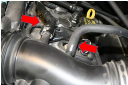
3. Loosen and remove two 4mm screws using 4mm hex wrench that secure the mass air sensor connection to factory intake.
