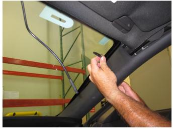
**Step 5:** Attach the two wires together and securely tuck them up above the headliner.
