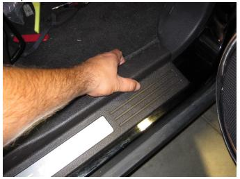
**Step 7:** Remove the kick panel by pulling out on the panel. Route the wiring down to this area. The wiring will be connected after the camera wiring is run.
