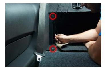
**Step 11:** Remove the (4) rear trunk trim retainers and remove the rear trunk trim from the car.
