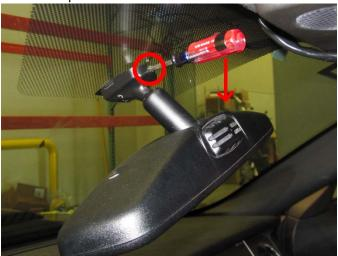
**Step 2:** Place the new mirror onto the windshield mount and tighten down the T20 torx screw until it isn't wobbly.
