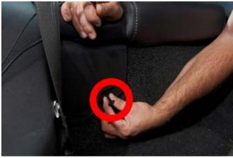
**Step 10:** Lay the rear seats down and run the wire back through the trim. Be sure the wires are clear of the rear seat hinges and pinch points. Remove these two push pins and route the wire behind them
