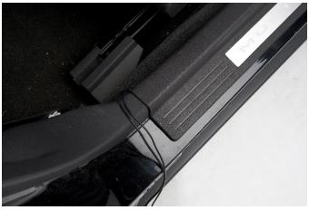
**Step 9:** Remove this push pin and route the wiring behind the trim panel. Press the wire down along the seats.
