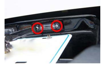
**Step 14a:** Pull down on the outside of the license plate light bulb retainer and feed the wire through it. Attach the camera wire to the intermediate camera wire inside the trunk. The license plate bulb retainer may need to be notched a little to keep from pinching the wire.
