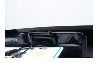
**Step 14b:** A hole can be drilled between the license plate lights to run the camera wire, if preferred.
