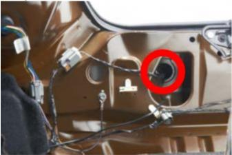
**Step 13:** Remove the (2) passenger side, license plate light bulb retainer screws.
