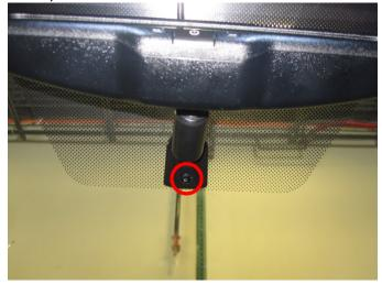
**Step 3:** Run the wires upward to the headliner. Place the included wire cover over the wiring. Clip it into the rearview mirror mount and extend it up to the headliner.
