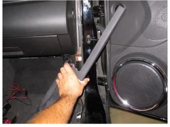
**Step 8:** Run the camera intermediate wiring under the step trim. Continue running the wire through the rest of the car.
