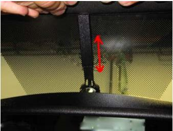
**Step 4:** Pull down part of the A plillar trim and run the intermediate mirror wire up from the kick panel to the rearview mirror wire.
