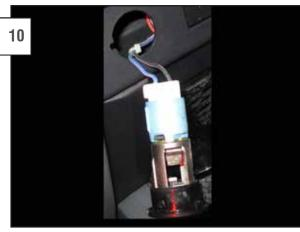
Make sure your 12V power outlet turns off with the key removed, then attach the red wire to the positive side and the black wire to the negative side using the supplied wire taps.
