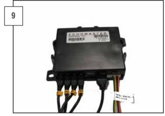
Plug the sensors, speaker and wire harness into the control module.
