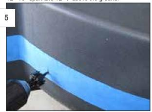
After careful measurement, drill a hole into the bumper. Run the wire harness behind the bumper and stick the ends out of the holes to insert the sensors onto.
