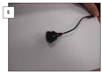
If the sensor placement is on an angle use the 6 or 12 degree inserts to correct the angle of the sensors so they are perpendicular. Place the sensors on the wire and press them into the bumper.
