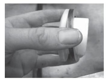
37. Reinstall the bushings, shims, and crush sleeves in the control arms.
