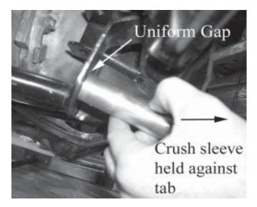
29. At this point, check the inner surface of each control arm mounting tab for weld spatter from Ford's production process. It is important that the mounting area of the Delrin be smooth to reduce friction. If any weld spatter is present, use a chisel or flat file to remove it.
