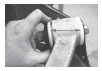
Note: There are four types of shims provided with each kit: Large diameter shims (thick and thin) for the large bushings, and small diameter shims (thick and thin) for the smaller bushings. More are provided for the smaller bushings since they will require thicker shim stacks.
