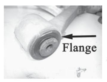
14. Place the large diameter press washer on the opposite side of the control arm bushing.
