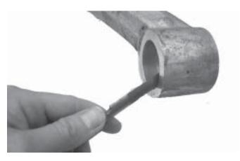
20. Using the supplied Scotch-Brite pad, remove any rust residue from the steel shell and smooth out any rough spots. When finished, wipe the area with a clean rag.
