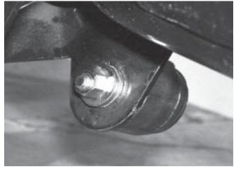
28. Tighten the bolt to pull the tab straight. Be careful to not over bend the tab. It may be necessary to move the setup around and repeat the process to flatten the entire mounting surface.
