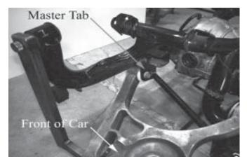
33. On all of the other bushings, open up a gap between the bushing shoulder and the control arm shoulder by pulling the bushings away from the arm, toward the mounting tab surface as shown.
