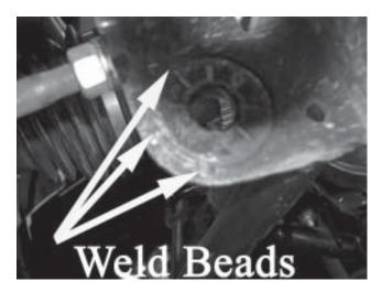
21. Using a small cut-off wheel attached to a drill or die-grinder, grind through the weld beads attaching the spacer to the tab. DO NOT grind deeper than necessary, the surface must be smooth for the MM delrin bushings to function properly.
