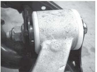
32. Push the arm against the "Master Tab." This is the tab that has a reinforcement tube welded to it. It is the front-most tab of the rear control arm mount. The arm will be pushed toward the front of the car. No shims are used at the Master Tab.
