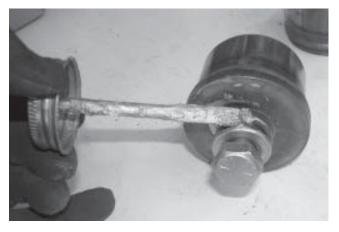
12. Apply anti-seize between the washers, the head of the bolt, and the removal cup.
