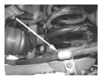
14. Make sure the parking brake is not set, then remove the parking brake cable housing retaining clip on each caliper.
