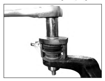
NOTE: It is possible that the nut will bottom out on the threads before the bushing is completely removed. If this happens, place additional 7/16" washers under the bolt head, or under the nut, and repeat Step 9.
