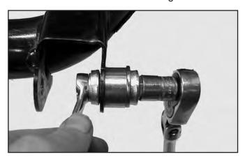
NOTE: To check tab straightness, set the crush sleeve flush against one tab. There should be a uniform gap from the crush sleeve to the tab at the other end. Continue the process until the tabs are straight.
