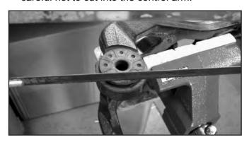
NOTE: There is an upper and lower part of the flange. Cut through both. The photo below shows a removed bushing with the flange properly cut.
