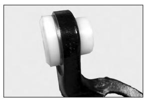
24. Install the crush sleeves and one 1-3/8" Diameter shim around each end of the crush sleeve as shown below. (Control arm removed for clarity)
