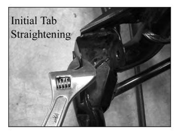
13. Set the Tab Straightening Spacer on the outside of the tab. Place the 3/8 G8 washer, 3/8 thick washer, and 5/8 G8 Washer on the 3/8-16 x 2" long bolt. Run the bolt through and place the other thick washer, 3/8 G8 washer, and nut on the inside of the tab. Use anti-seize compound or grease on the threads and washer surfaces.
