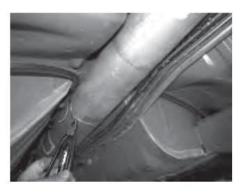
13. Unbolt the parking brake cable mounting-bracket from each control arm.
