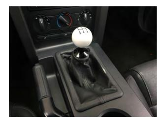
Then thread the shift knob on until it stops. Back the shift knob off so that the shift pattern is aligned properly. Then turn the retainer counter clockwise until it locks against the shift knob.
