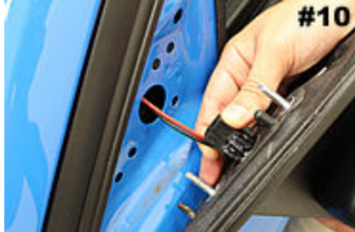
Lamp wiring goes through same hole as the mirror's electrical connector.
