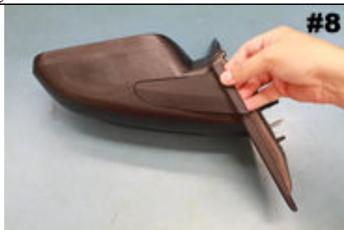
Remove the rectangular access cover on the bottom of each mirror.
