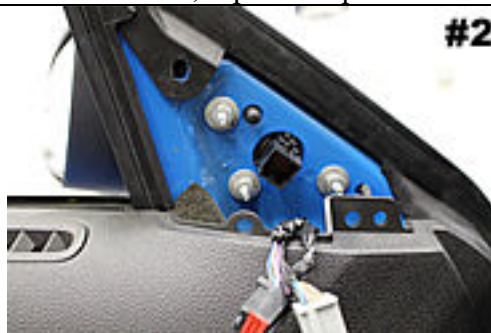
Remove the 3 - 11mm nuts holding mirror on. Don't drop the nuts!
