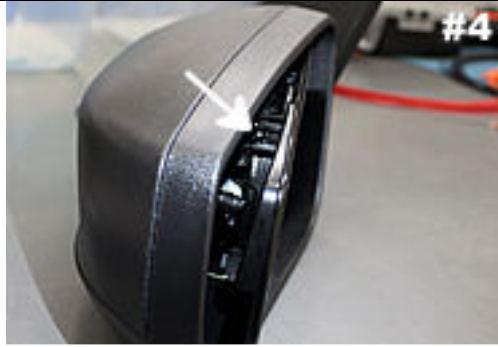
Shows top retaining tab. Insert flat head screw driver here to release tab.
