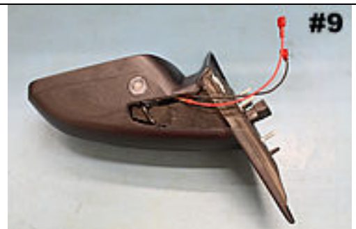
Mount the lamp using the white nut provided, then route wiring as shown.
