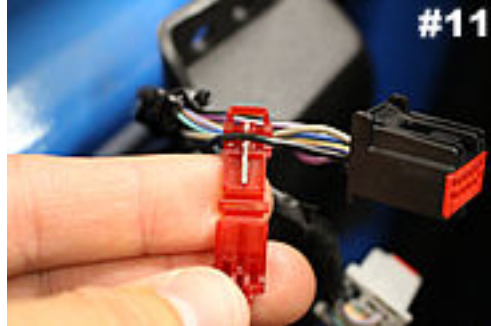
Slide wire into place and close wire tap firmly.
