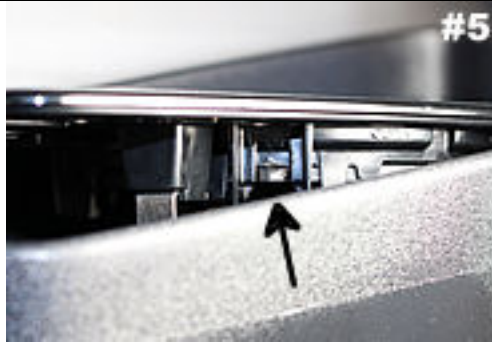
View of Drivers side mirror, bottom. Outboard (left) retaining tab.
