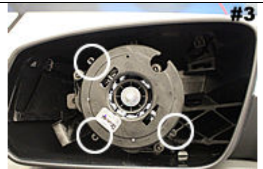
3 Retaining tabs (circled) hold the mirror glass in place.
