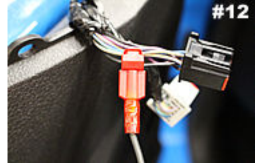
Plug correct wire into the wire tap as indicated in manual.
