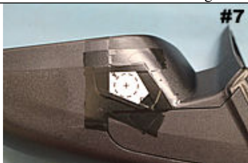
Bottom of driver side lamp with drilling template attached.
