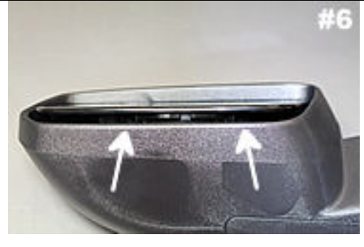
Bottom view of Drivers side mirror. Arrows point to 2 of 3 retaining tabs.
