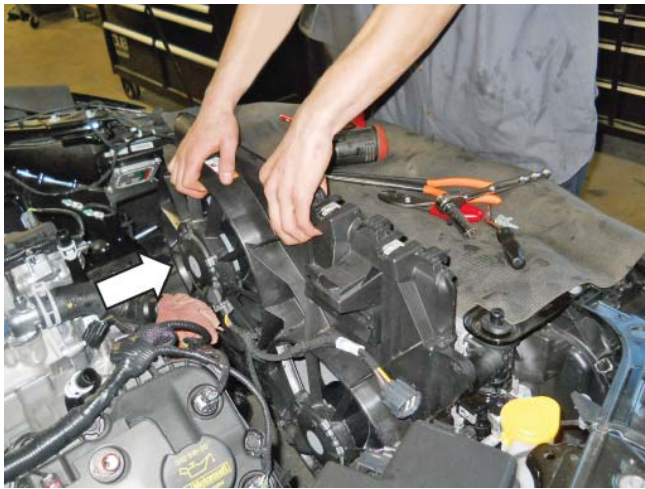
51. Remove the three (3) bolts securing the water pump pulley to the engine and remove the water pump pulley.
