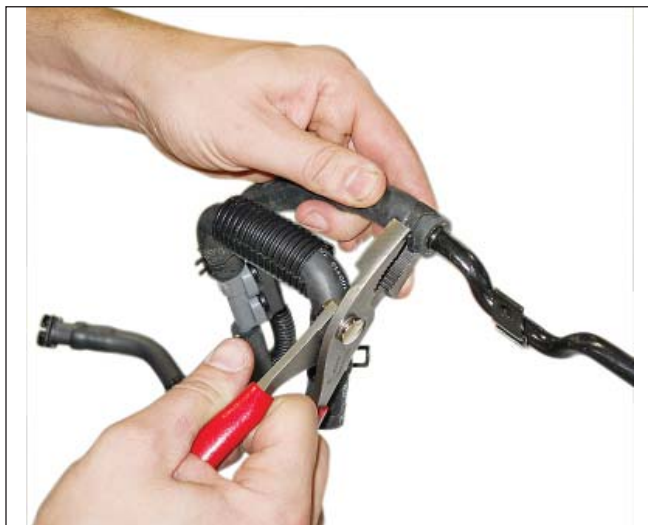
9. Release the clamp and separate Section B, hose 2, from the steel tube.
