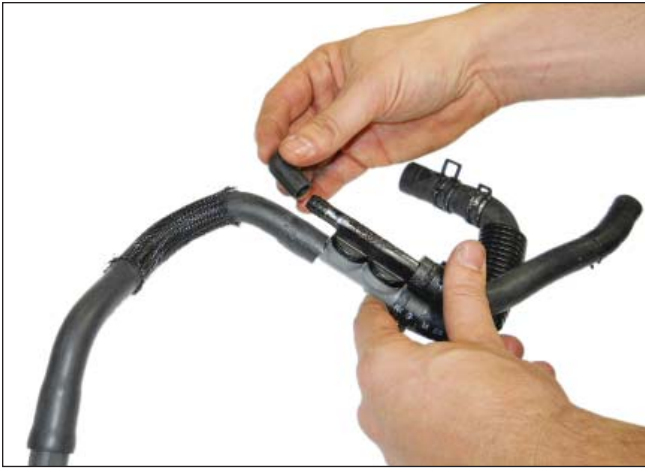
13. On hose 4, remove the convolute off of the curved end.
