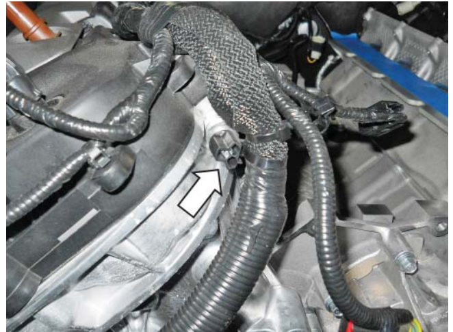
53. Unclip the engine electrical harness retention clips that retain the engine harness to the top corners of the RH (passenger side) front cover.
