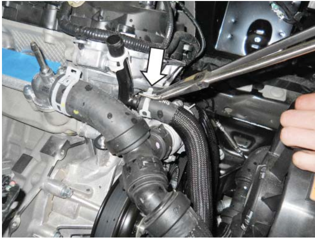
Degas hose from bottom of bottle
