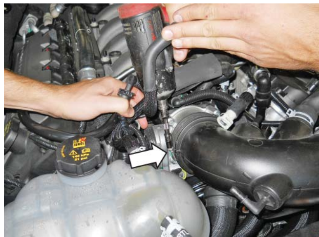
Clamp at throttle body
