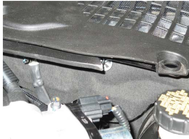
Exposed point on modified K-brace, shown installed
