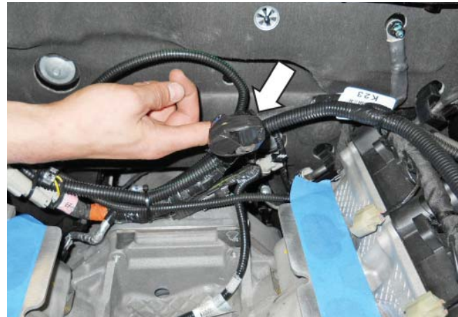
CMCV connectors taped up
