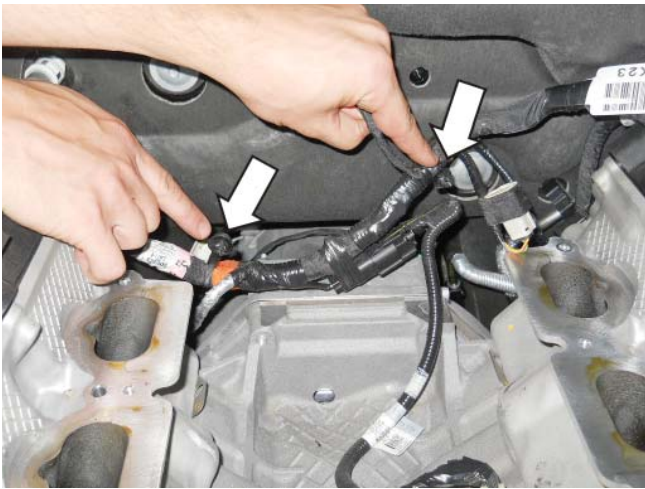
Pin retainers on harness
