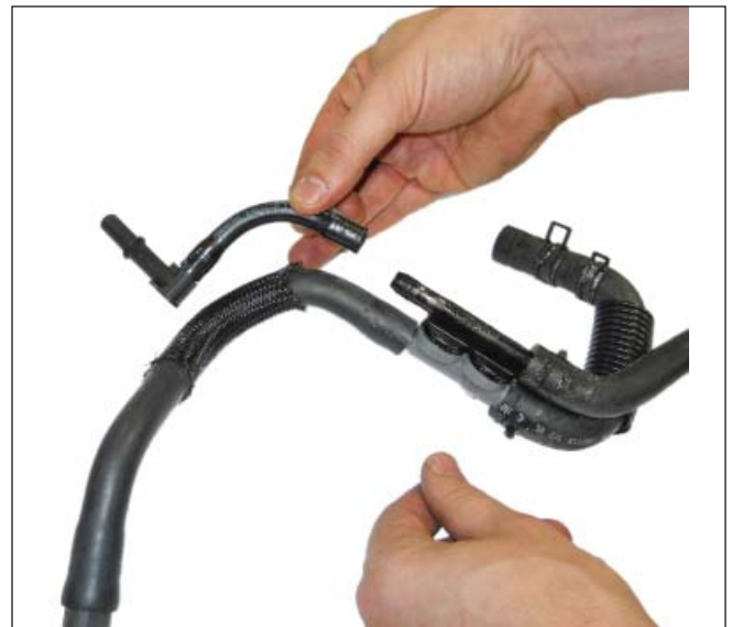
12. Install the Cap Plug (CS2575) found in Hardware Kit D (1315-TVSHKD) on the now open port of the brake aspirator.
