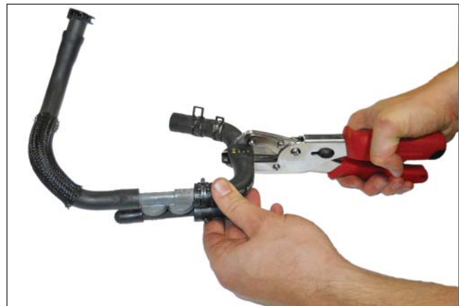
16. Remove the dual clamp from the severed hose. Cut the clamp in half to become a single clamp. Trim the excess metal. Transfer the single clamp to the remaining hose end.
