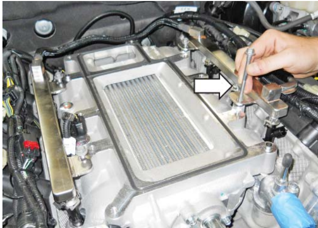
8. Connect the eight (8) fuel injector electrical connectors.
