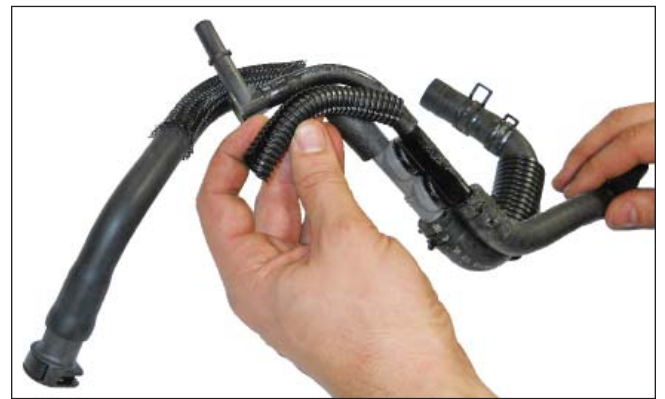
11. Cut and remove the curved nylon tube from the brake aspirator.
