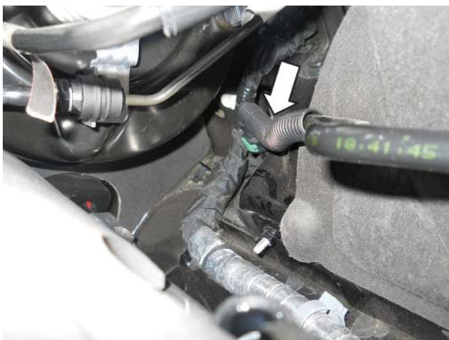
Disconnect green quick connect fitting
