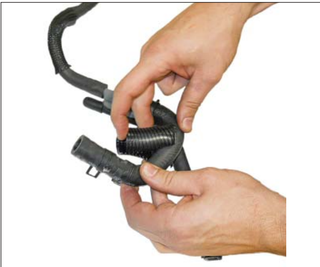
14. Loosen the clamp and rotate the curved hose (hose 4) end 180 degrees. Reinstall the clamp.
