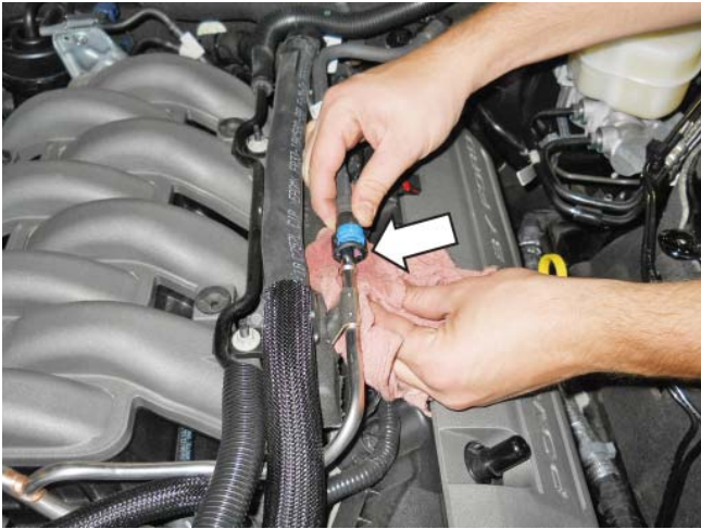
29. Disconnect the brake booster vacuum hose from the intake manifold. This port is located directly behind the throttle body.
