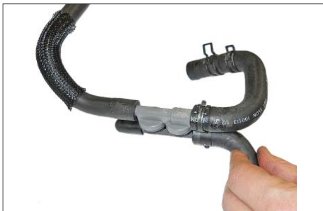
15. On the hose just rotated, mark a line 2" from the bend coming from the aspirator as shown, and cut the hose.
