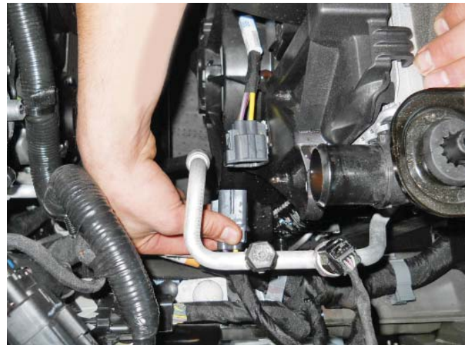
Fan shroud electrical connector
