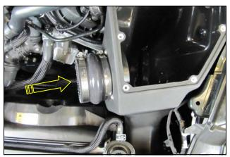
**9.** Slide the Hump Hose and Clamps onto the Filter Adapter as shown. Do not tighten the clamps at this time.
