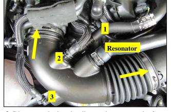
**3.** Disconnect the breather lines and resonator tube from the intake. Depending on your configuration, you may have two or three lines. Loosen the hose clamps and re-
