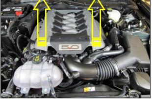
**2.** Remove the strut tower brace is so equipped. Lift up on the engine cover to unseat it from it's mounting grommets and set it aside.
