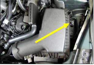
**5.** Remove the 6mm airbox mounting bolt in the inner fender and lift the entire airbox assembly out of the vehicle. Set the bolt aside for now. It is to be reused.
