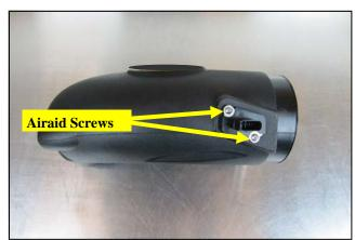
**14.** Insert the Mass Airflow sensor into the Airaid intake tube as shown and secure it suing the #8 Button Head Screws. Do Not Use the OEM hardware.
