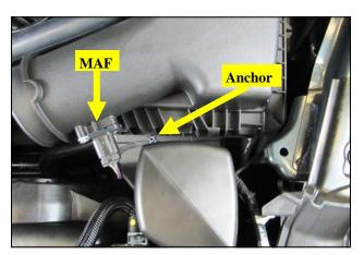
**4.** Gently pry the harness anchor out of the airbox and disconnect the mass air flow meter.
