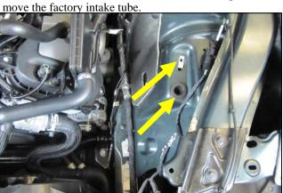
**6.** Be sure the speed clip and the airbox grommet remain inside the vehicle. They will be reused.
