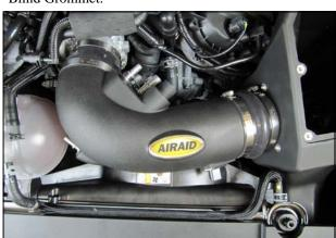
**15.** Insert the Intake Tube into the Hump Hose and Reducer then tighten all 4 Intake Clamps. Apply the Airaid Decal onto the Tube as shown.
