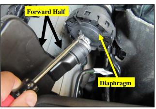
**11.** Using a standard screwdriver, carefully pry open the clamp on the resonator diaphragm and remove the forward half of the resonator.
