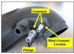
**12.** Insert the Grommets and Aluminum Fittings into the Airaid Intake tube as shown. On vehicles not equipped with the small breather, plug the hole with the Blind Grommet.
