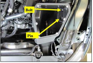
**8.** Place the Airaid Airbox assembly into the engine compartment as shown, with the locator pin on the bottom of the box inside the fender grommet. Secure the Airbox by reusing the 6mm bolt removed in step # 5.
