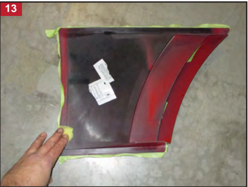
STEP 13: Make sure the painters tape is removed from the 3M tape areas, then apply 3M adhesion promoter to the areas.
