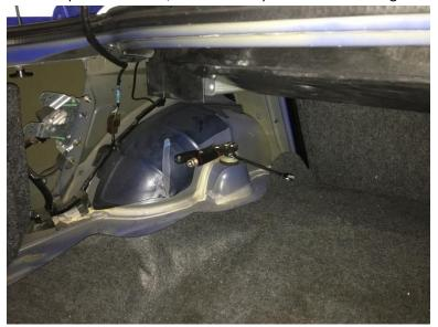
**4.** Before removing the 15mm nut completely, raise the rear end slightly with a floor jack.
