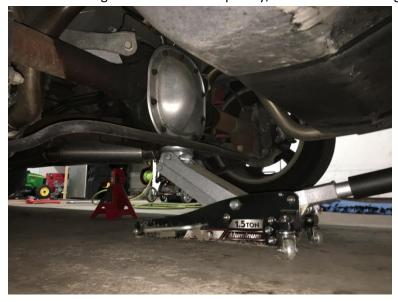
**5.** Loosen and remove the lower shock mounting bolt using a 15mm and 18mm socket. Then finish removing the upper mounting nut and remove the shock.
