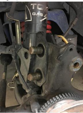
**8.** Before removing the two lower strut mounting bolts, place a jack under the lower control arm. With bolts removed, separate the spindle from the strut.
