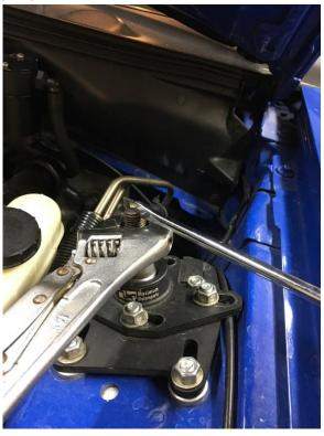
\*Note: if caster/camber plates are installed, keep track of the number of spacers between the spherical bearing and nut.
