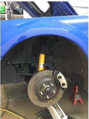
**16.** Reinstall the front wheels and torque lug nuts to 100 ft.-lbs.
