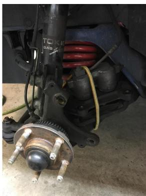
**6.** Remove ABS cable bracket by removing 15/16" jam nut.
