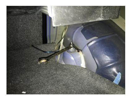
10. Your new KONI Sport adjustable shocks and struts are now completely installed. Lower the vehicle from the jack stands and use the adjustment knob included with the kit to set the damping to your personal preference.
