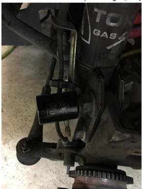
7. Remove 15/16" nuts from lower strut mount bolts using a 15/16" and 21mm socket.
