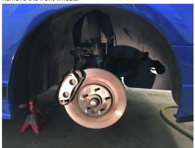
**4.** Loosen, but do not remove the upper strut nut using a 21mm socket and impact wrench, or flat blade screw driver and an open-end wrench. Certain setups may require a 15/16" wrench instead of a 21mm.
