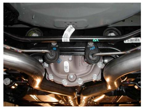
12. Reinstall rubber hangers removed from step #6 above, using (2) 8mm bolts.
