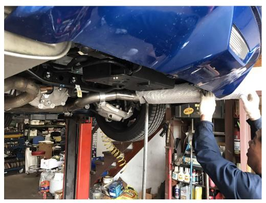
Slide the inlet pipe through on both end, engage inlet pipe hanger pin into the factory hanger then tighten the hanger back in place, slide Magnaflow muffler hanger pin into factory hanger.
