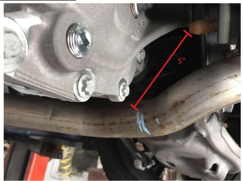
It's 5 inches from the factory pipe hanger pin end to a straight pipe portion where the cutting point lines up to the rare differential.
