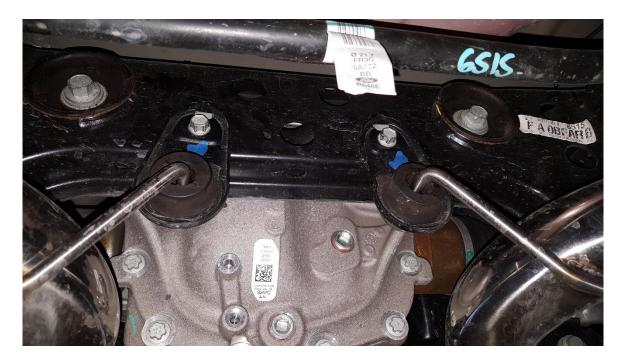
4. Bolt the differential pipes to the mid-pipe with the fasteners and gaskets.
