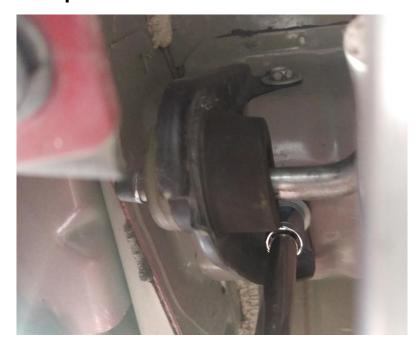
5. Remove factory exhaust by lifting upward and pulling toward the rear of the car until the mid-pipe/resonator is free from the front of the exhaust system.
