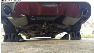
2. Loosen the 4 fasteners at the front of the mid-pipe.
