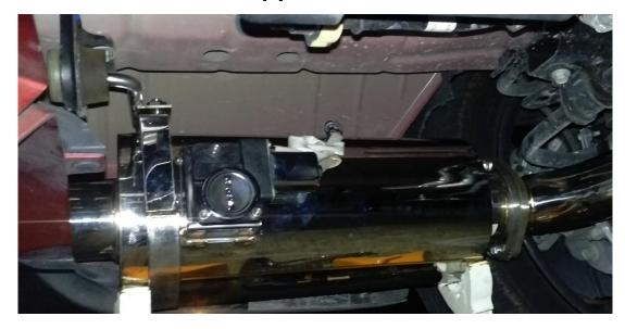
8. Install the tips onto the mufflers using a 6mm hex key.
