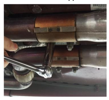
3. Remove the bolts securing each of the 2 exhaust hanger brackets to the frame just behind the rear differential.
