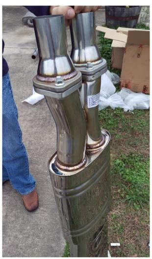
2. Insert the reducers into the connections you removed the old system from. (I used a rubber mallet to make sure they slid in all the way.) Place a jack stand under the mid-pipe to support it while you work on the rest of the system.
