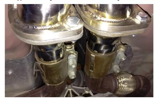
3. Reinstall the 2 exhaust hanger brackets onto the sub-frame behind the differential. Insert the hangers on the differential pipe sections into the brackets.
