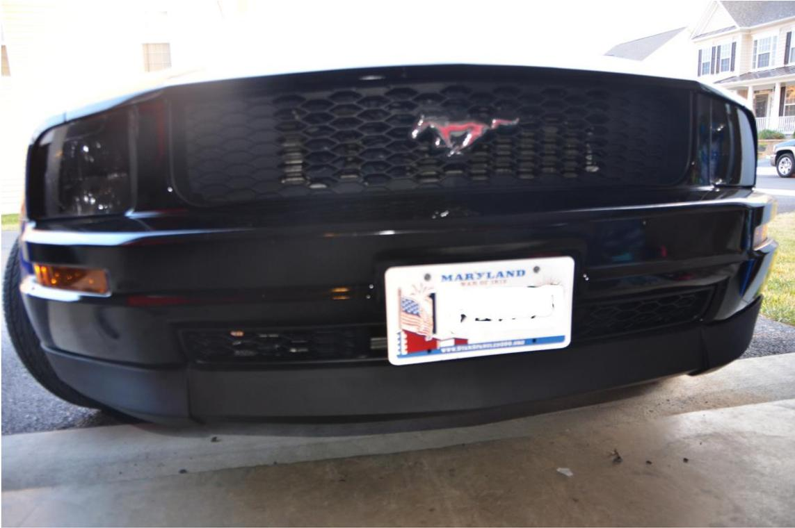
7. Install the two upper screws in both sides of the wheel well and tighten all four screws.
