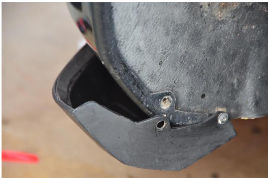
5. Gently pull the front of the MMD Chin Spoiler down and pull the cover off the double-sided tape that was preinstalled on the spoiler. Spoiler should not need to be pull down much further than shown in the picture below.
