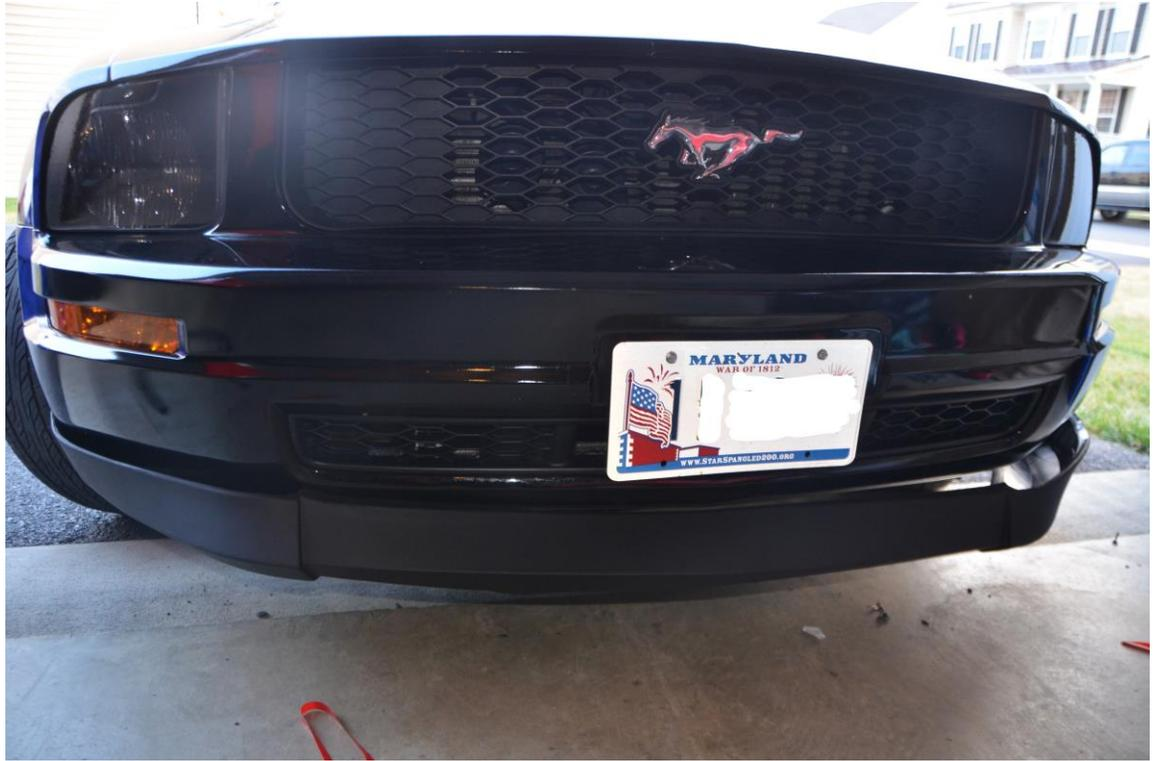
6. Once all of the tape covers are removed, line up the MMD Chin Spoiler with the bumper. Carefully position it in the final desired location and firmly press against the bumper.
