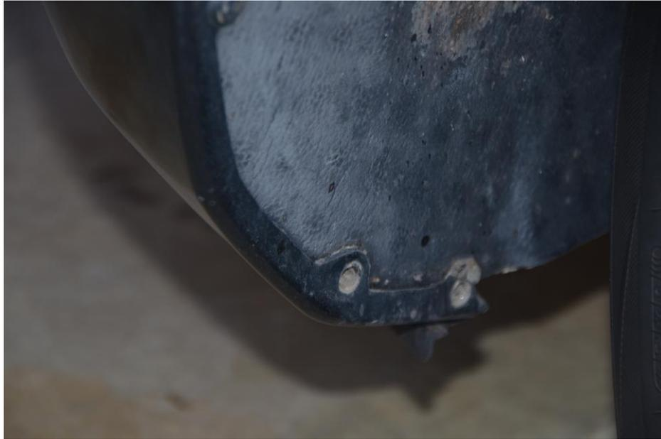
4. Position the MMD Chin Spoiler against the front bumper in the desired installation location. While holding the spoiler in place, install the two lower screws that were removed earlier to both sides of the vehicle. Do not tighten the screws at this time. This will hold the ends in place while you finalize the spoiler's position.
