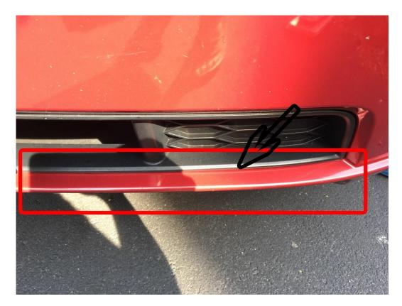
4. Pull up a few of inches of red covering from the 3M tape. You can do this from the side or middle and make sure to pull up a good amount. The goal of this is to be able to align the chin spoiler with most of the tape covered, and then pull off the rest of the tape covering, once the chin spoiler is in place. (Note: the chin spoiler is shown upside down here. The tape will be on the top when placed on the car).
