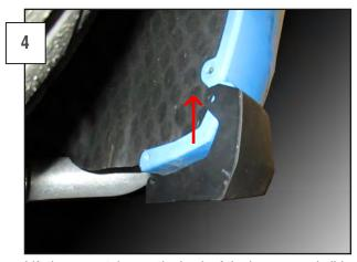
Lift the upper tab over the back of the bumper and slide the chin spoiler into place. Reinstall the (4) stock scews removed in step 1.
