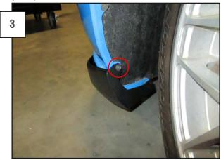
Install a screw through the top hole of the chin spoiler into the bumper and place the front of the chin spoiler over the front of the lower bumper, then move to the opposite side of the car.
