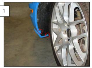
Turn the tires toward the opposite side of the car and remove the (2) phillips lower bumper screws, repeat this on the opposite side. Clean the bumper in front of the lower grill with the supplied alochol pad.
