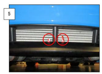
Make sure the chin spoiler is placed correctly and carefully pull the red 3M flags, until all the tape backing is removed, to expose the adhesive, then press the spoiler onto the bumper.
