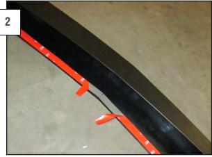
Pull up 2" of red 3M backing and fold them as shown; so they can be accessed from the front after installation. (The chin spoiler is shown upside down in the photo)
