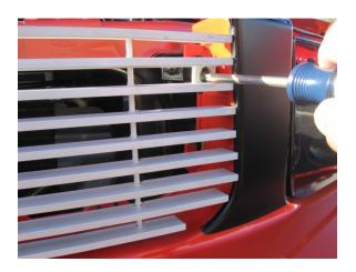
**Step 7:**Re-install the radiator cover removed in Step 1 to complete the installation.
