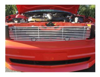
**Step 6:**Use the supplied screws to secure the billet grille to the brackets as shown.
