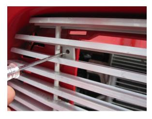
**Step 4:** Remove the billet grille and drill the marked spots using a 3/16" bit as shown.
