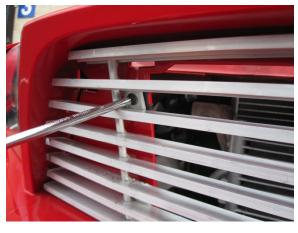
**Step 6:**Re-install the factory radiator cover and clips removed in Step 1 to complete the installation.
