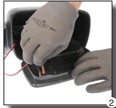
Fig. 2. Reconnecting the mirror glass assembly.
