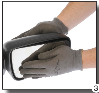
Fig. 3. Installing your new mirror glass assembly.
