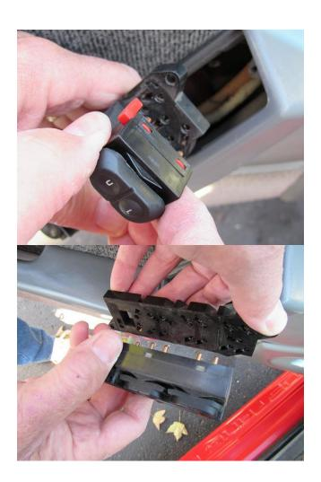
(NOTE: The door lock switch has a red tab at its upper left that corresponds with an opening in the switch plate. The window switch has a rectangular tab at its bottom that corresponds with an opening in the switch plate.)
