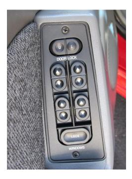
(Tip: The black finish had been worn off the original bezel screws in my Mustang. I took the original screw to my friendly local Ford dealer. Apparently these screws have been used for many years and are an in-stock item. The new screw restores the original factory finish look.)
