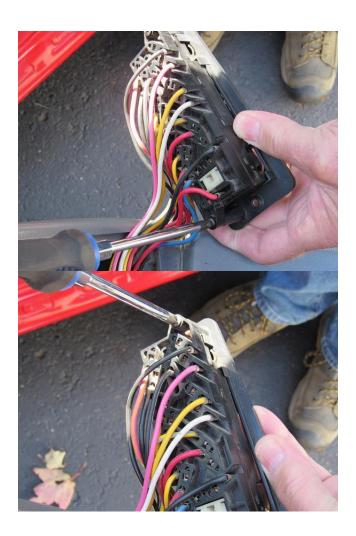
3. The switch assembly is simply lifted away from the bezel
