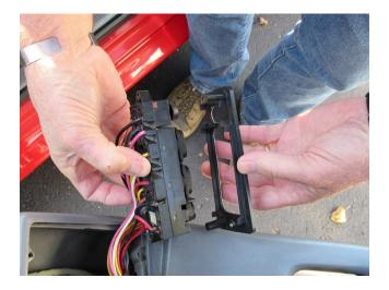
4. The power lock switch and window switches are simply pulled off the connector with your fingers. You will probably have to wiggle the switch bases a little bit to get them to come loose.
