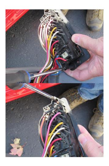
3. Place the reassembled switch bezel back into the opening in the door panel. (No force is necessary, it should simply slip in.)
