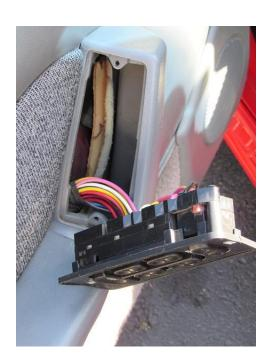
2. The switch assembly is held to the back of the switch bezel by two Phillips screws. Remove them and set them aside.
