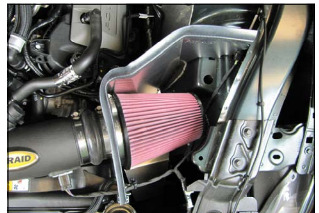
21. Install the Airaid Premium Filter onto the Filter Adapter. Install the weatherstrip on top of the Panel assembly as shown with the contour rolling away from the filter.
