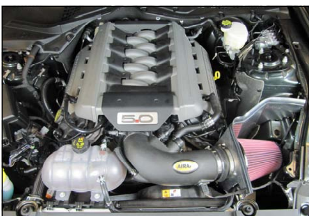
22. Double check your work. Make sure all clamps, hoses, bolts, and screws are tight. Double check the hood clearance. Reconnect the negative battery cable and reinstall the cover and strut brace, if so equipped.
