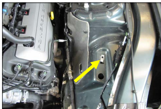
7. Be sure the speed clip remains inside the vehicle. It will be reused.
