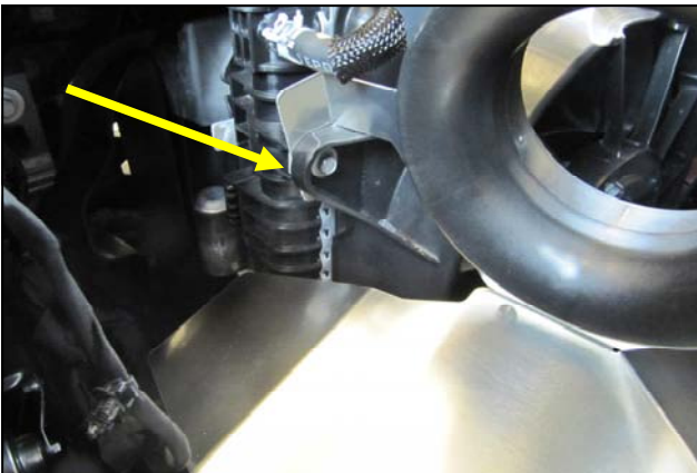
13. When properly installed, the Panel tab resides behind the fan shroud as shown.
