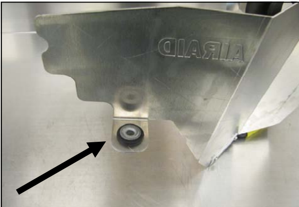
8. Transfer the OEM air box grommet and anti-crush sleeve into the Panel assembly as shown.
