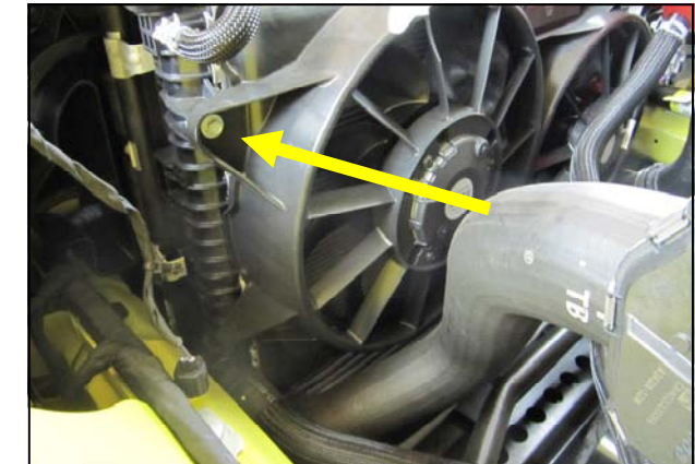
9. Remove the drivers side fan shroud bolt and set it aside.
