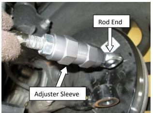
**Step 5** Insert the tapered end of the tie rod stud into the spindle and tighten it using the supplied hardware. After insuring that the wheel is still centered and after tightening the tie rod stud you will need to adjust the Gripp Adjuster Sleeve so the outer tie rod end lines up with the rod stud. Once proper alignment is achieved tighten the Jam nut.
