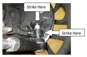
**Step 3** Remove the outer tie rod by using one wrench to hold the Jam nut and another wrench to turn the tie rod. Once the jam nut is broken loose, keep the wrench on the inner tie rod and thread the outer tie rod off.
