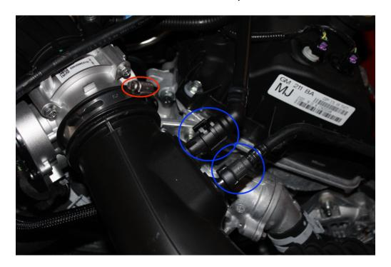
7. Now remove the clean air tube. This completes part one of the installation.
