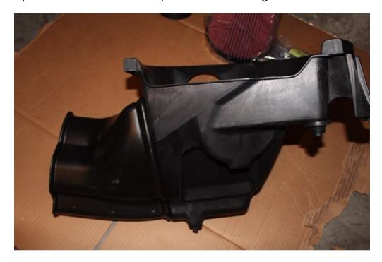
4. Place this assembly where the stock air box was before removal. The rubber fittings should align in the vehicle, and the 10mm bolt can be used to secure the box. It should only be hand tightened to approximately 6 ft-lb:
