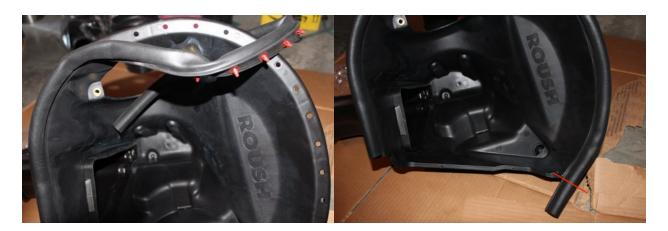
3. Attach the Dirty Air Inlet (2) to the Roush Air Box (1). The two pieces slide into place and no tools are required to fit them together.
