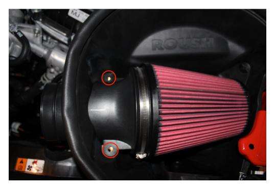
7. Connect the Clean Air Tube (6) between the Filter Tube (3) and the throttle body. The result is shown in the picture below. Tighten the clamps circled in red, and replace the hoses in the nipples circled in blue.
