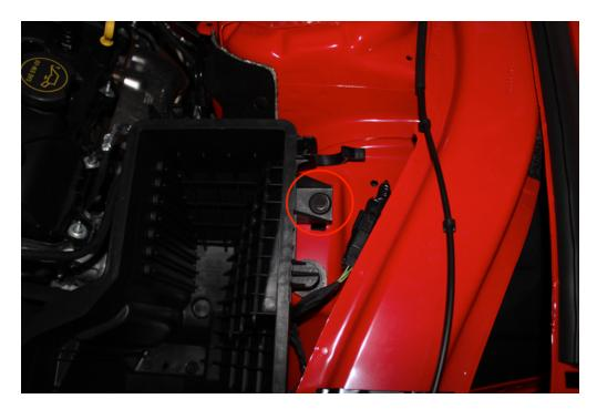
4. With the bolt removed, the stock air box can be removed altogether. Lift upwards as you shimmy and wiggle the box to loosen it. This is what the air box looks like after it is removed:
