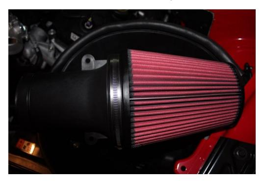
6. Put the filter and tube assembly into the Roush Air Box (1). The tube side should be placed through the air box from the inside outwards. When aligned correctly, the two 10mm Bolts (5) can be used to secure the filter to the air box. They should be hand tightened to approximately 8 ft-lb. The bolt locations are circled in red in the picture below.
