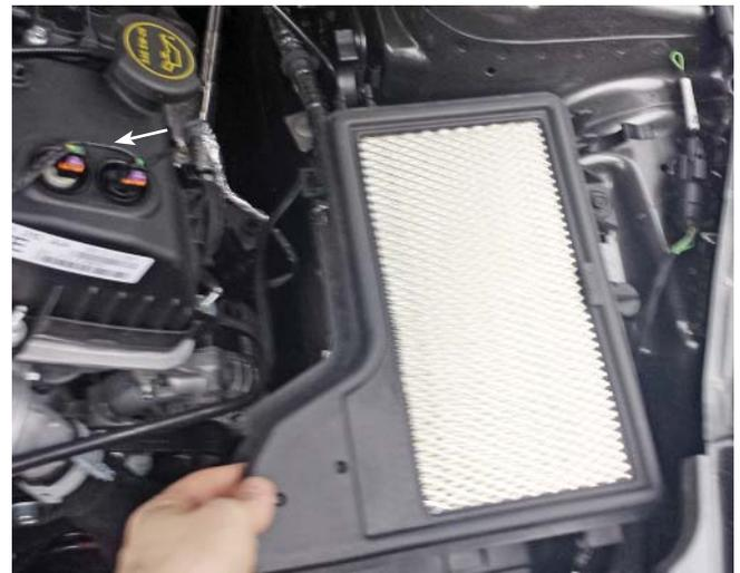
6. Using the 10 mm socket, remove the bolt holding the air box to the inner fender. Retain the bolt as it will be used during installation.
