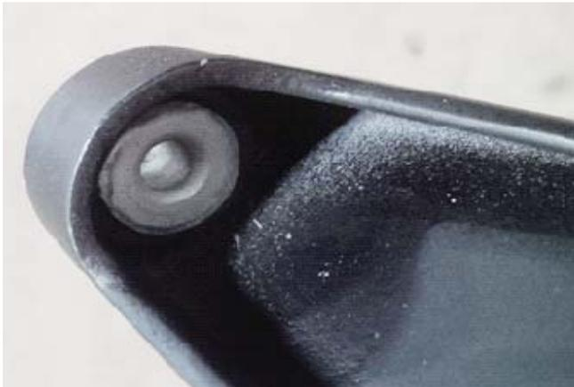
2. Install the second grommet onto the air box (P/N: 131550-9A612).
