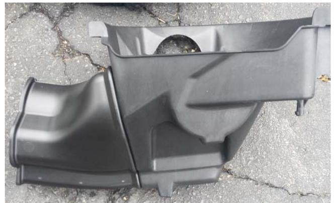
5. Place the bulb seal (P/N: 131550-9C664) onto the top of the air box (P/N: 131550-9A612) and clip into the holes. Trim ends as required.
