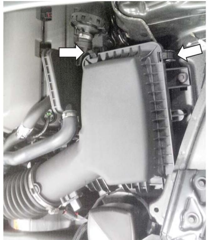
5. Remove the air box lid and filter. Retain the lid for use during installation.
