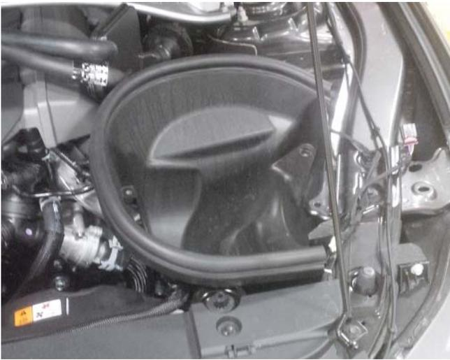
7. Using a 10 mm socket and the bolt removed from the stock air box, attach the air box to the vehicle. Torque to 8 Nm.
