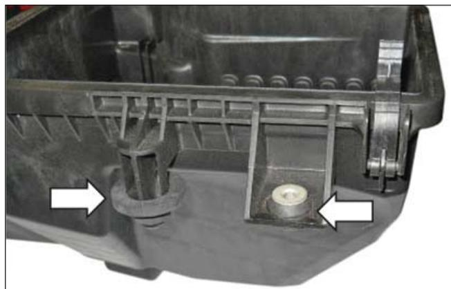
11. Remove the rubber isolator from the bottom of the stock air box tray and retain for use during installation.
