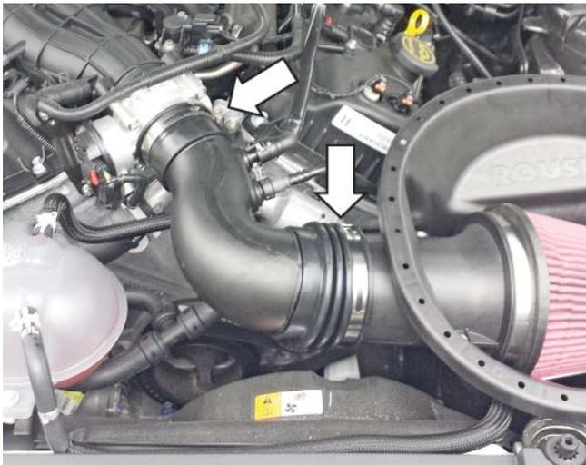
11. Connect the two (2) quick connect fittings previously removed to the new clean air tube.
