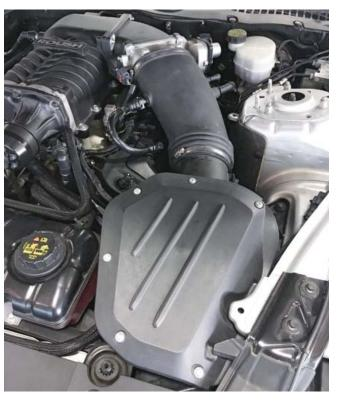
Begin by loosening the hose clamp where the clean air tube connects to the throttle body.
