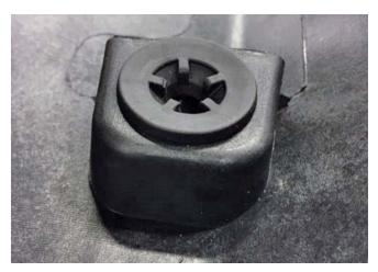
2. Installation to the valve covers is the reverse set of operations from the removal of OEM covers. The "Fingers" on the coil cover point inboard towards the center of the engine. Notice the features unique to each coil cover. The driver side coil cover shown below has a large semi-circular notch on the bottom; the passenger side has a notch for the oil fill cap by the front.
