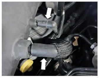
5. Pull the clean air tube towards the front of the vehicle, compressing the bellows near the air filter housing. This will allow the opposite end to come free from the throttle body. Once free, simply lift the clean air tube up and out.
