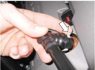
2. Pull up firmly on the OEM coil cover to remove it from the valve cover retaining studs.
