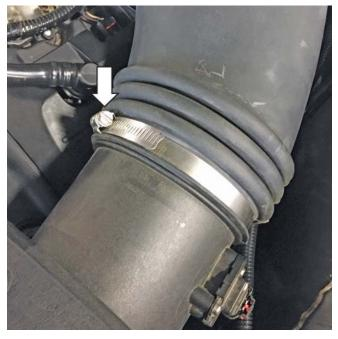
3. Remove the PCV hose from the valve cover and from the clean air tube. Push the gray tabs clockwise as shown and pull firmly to remove.
