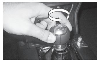
Inspect the threads on the shift-lever for debris and remove any if found. Clean the oils off the threads using Brake Cleaner or equivalent cleaning agent and allow the agent to dry/ evaporate.
