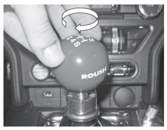
Screw the shift ball down until the bottom of the ball sits lower than the top of the positive lockout, and then continue to turn clockwise until the shift pattern on the top of the ball rests in the desired position.
