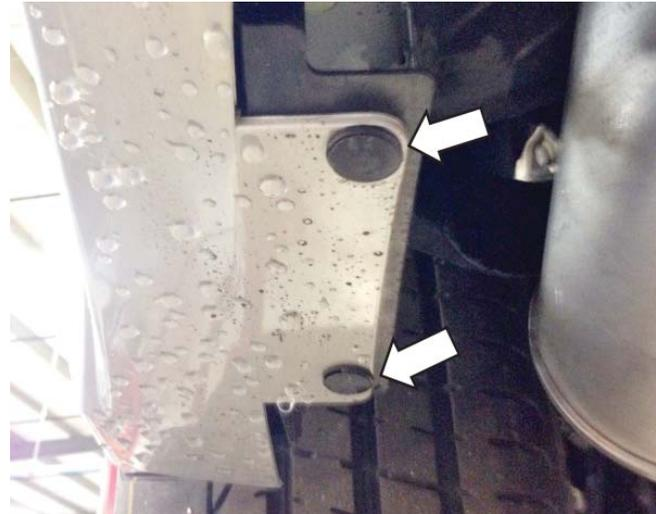
6. Remove two (2) 7 mm screws and two (2) push-in retainers on the LH and RH sides under the rear bumper.
