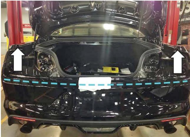
9. Locate and release one (1) retaining tab on each side of the bumper cover near the outer edge of the tail lamp mounting area.
