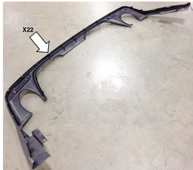
22. Using an air saw, cut and remove the factory lower valance as shown below.
