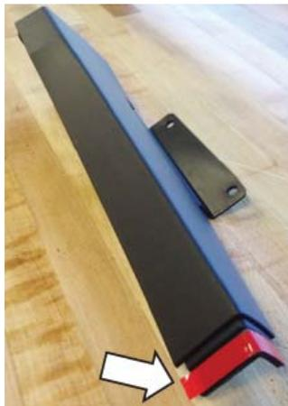
34. Install three (3) J-clips that were removed in step 17 onto the side valance pieces as shown in next image and create a removal tab with a portion of the 2-sided tape backing.
