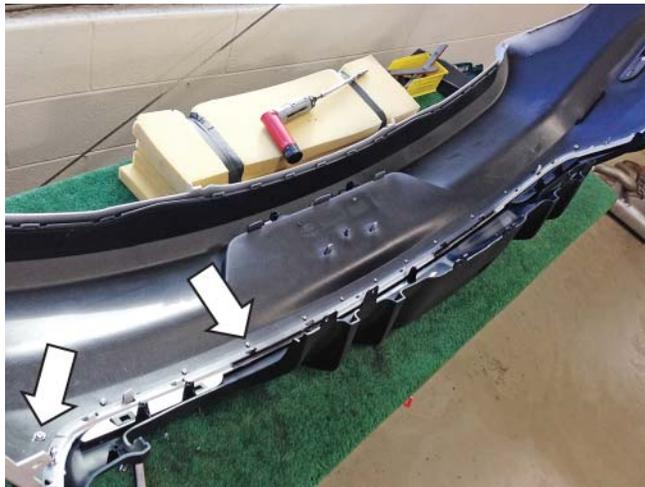
33. Apply 3M Ad-Pro® (P/N: 021200-27571) onto the rear edges of the side valance pieces (P/N: 1315-17F955 & 1315-17F956) and then install the 2-sided tape (P/N: TAPE-015-12.5x68).
