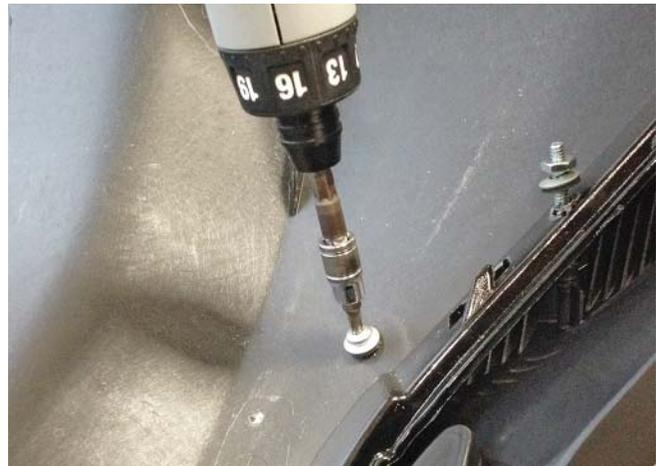
32. Remove the backing off the 2-sided tape, apply blue Loctite® to the threads on the studs that were installed in step 24 and then torque all of the fasteners that were installed in steps 24-26 to 0.7-0.8 Nm.
