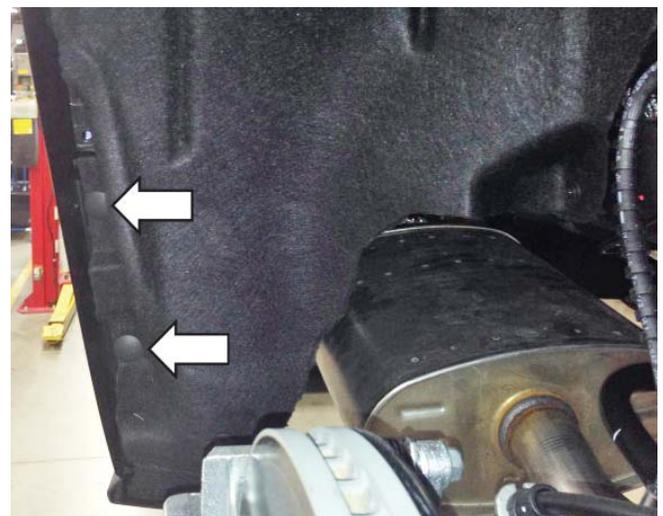
4. Pull the inner rear fender covering back to reveal the three (3) screws and remove them with a 7 mm socket.
