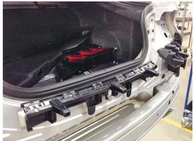
11. Disconnect the side marker electrical connectors as well as the edge clips that retain the wiring harness on each side of the bumper cover.
