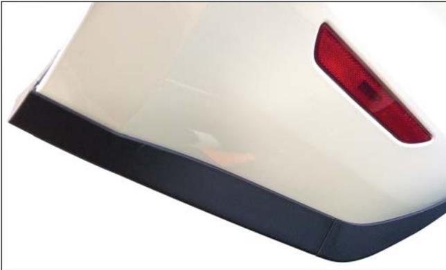
36. Reinstall the rear reflectors, reverse light and the bumper cover reinforcement piece that were previously removed by reversing steps 14-16. Reinstall the side marker, license plate light, trunk release and reverse light electrical connections that were previously removed by reversing steps 11-13. If equipped reinstall the factory back up sensors into the new brackets that are on the ROUSH rear valance (P/N: 1315-17F954BUS).
