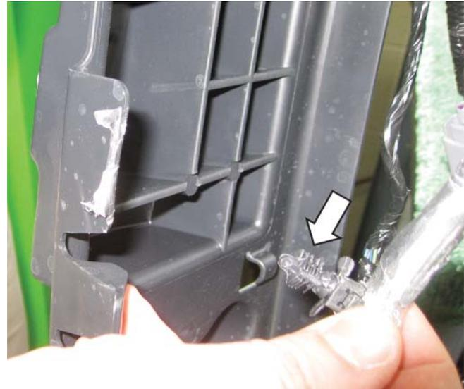
38. Drill a 1/4" hole as shown below, reinstall the push-in retainer and then trim the excess.
