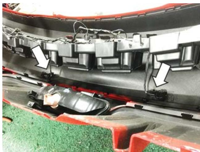
17. Remove the four (4) factory back up sensors by releasing the retaining tabs and then set them in a safe place. Remove the four (4) plastic factory back up sensor brackets from the bumper cover with a suitable cutting tool. Use caution to not damage the factory bumper cover.
