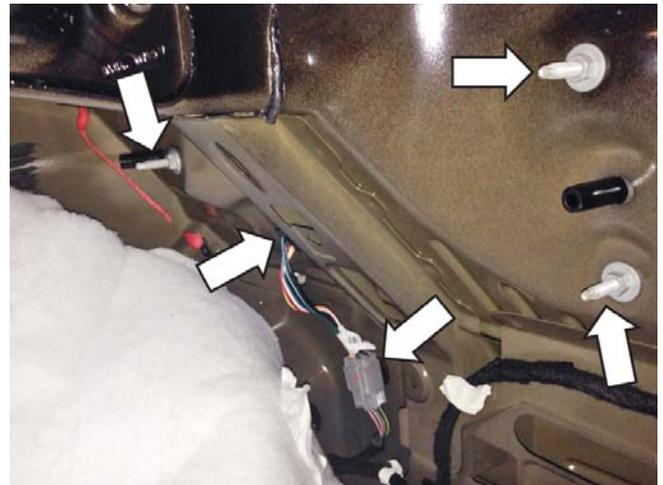
3. Remove three (3) push-in retainers in the back of both rear wheel wells.
