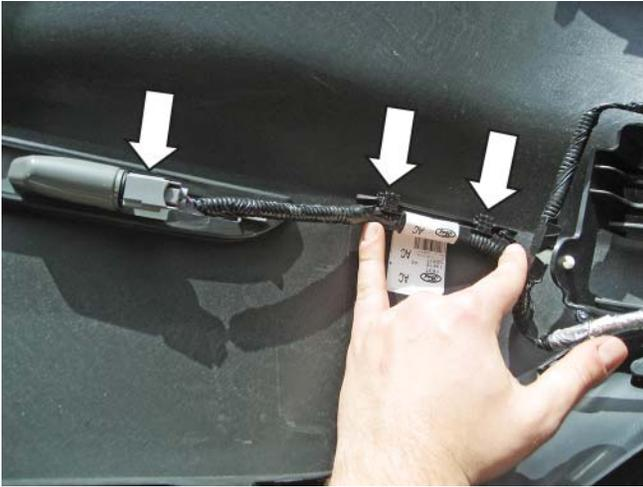
12. Disconnect the license plate light and trunk release electrical connectors as well as the two (2) edge clips that retain the wiring harness.
