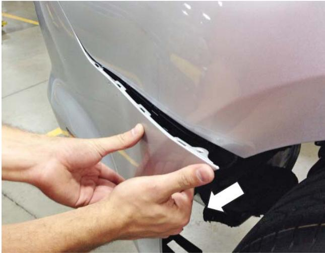
8. Pull up and rearward along the top edge of the bumper cover to release the upper retaining clips.
