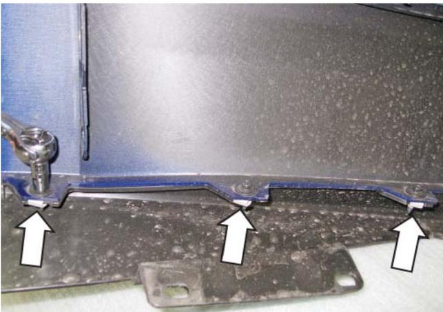
21. Remove the lower bumper cover trim piece by releasing the twenty-two (22) retaining tabs.
