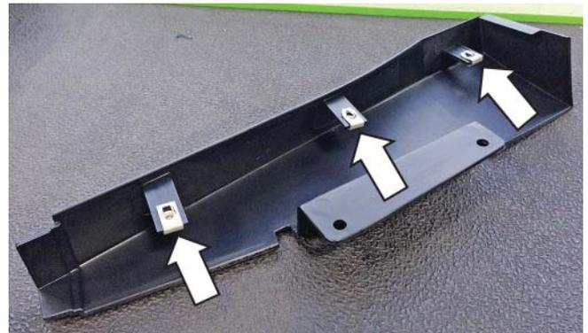
35. Install the side valance pieces onto the rear bumper cover using three (3) screws that were removed in step 17 and completely remove the backing from the 2-sided tape. With the side valance pieces installed press firmly along the back edges to ensure that the 2-sided tape has bonded adequately.
