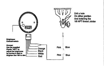
You will need to drift and top a 1/6th NPT fitting for the probe to go into. We recommend a professional to tap this. Try to avoid shavings from going into the manifold or exhaust.
