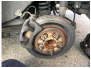
Using 13 mm socket remove caliper sliding bolts. (Circled in red) slide caliper pins back and forth feeling for any resistance, if a little resistance is present pins should be lubecated and if the pins have a lot of resistance present replaced with new ones and lubercated.
