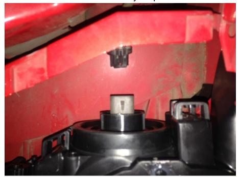
5. Next, position the headlight housing so that you can disconnect the parking light wiring harness. There is a clip on each side that you can lift up on and disconnect the harness. The clips can become very brittle so be careful not to break them.
