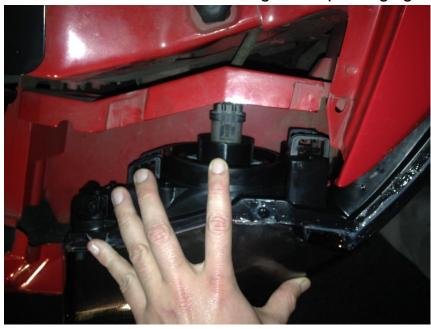
4. Once you have pulled the head light assembly away from the car and exposed the wiring harnesses, detach the headlight wiring harness by pulling it straight back from the headlight housing. Note: Using a small flat head screwdriver may help release the retaining clip.
