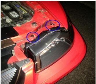
3. Carefully start to remove the headlight assembly by pulling straight to the front of the car. Be careful not to pull too hard because there may not be much slack in the headlight and parking light wiring harness.
