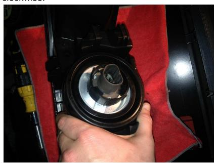
8. Remove the stock headlight bulb by firmly pulling straight out of the housing. Once removed set aside as it will not be reused.
