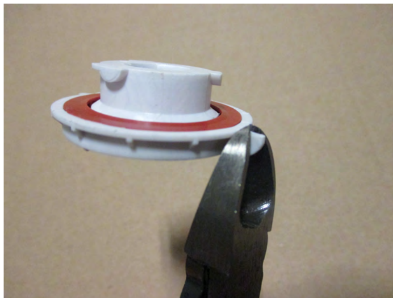
Step 3// Using cutters, cut the tabs flush with the outer ring.
