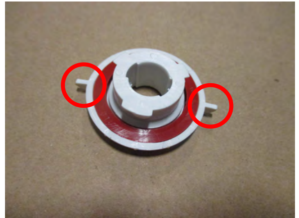
Step 2// Locate the protruding tabs that are causing interference with the headlight housing.
