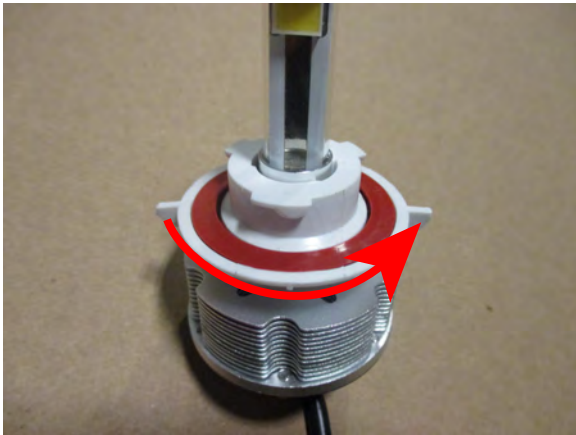
Step 1// Remove the white plastic retainer.
